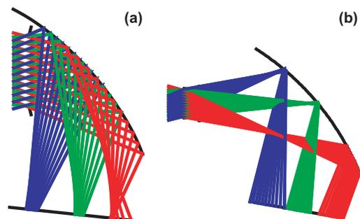
FIG. 4. (Color) Ray tracing results to find the optimized shape of the mirrors: (a) Optimized M1 without L1. (b) Optimized M2 without L2.
