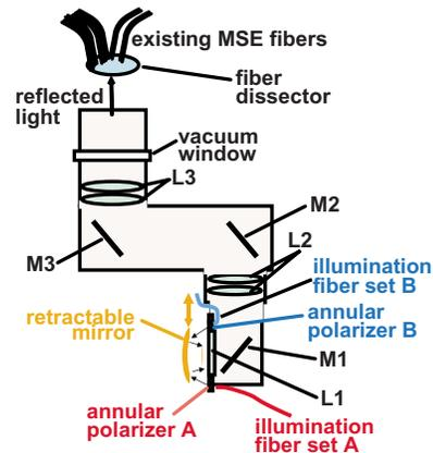
FIG. 5. (Color online) Proposed layout for an *in situ* calibration system for MSE on Alcator C-Mod. Linearly polarized light strikes a mirror that is slid in front of the plasma-facing lens (L1) shortly before and after a shot.
