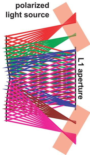
FIG. 6. (Color) Ray tracing calculations to optimize the retractable mirror shape to provide the full MSE field of view at all angles. The rays with different colors simulate those from the real light source from the beam from different channel locations.
