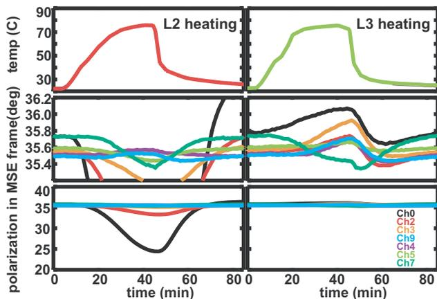
FIG. 2. (Color) In-vessel canister heating test results. The plots on the left column are for the L2 heating test and those on the right for the L3 heating. The top plots show the temperature variation over the experimental time. The second plots are the magnified version of the bottom plots. The channel numbers are written in the order of the tokamak major radius (Ch0, edge most; Ch7, core most).
