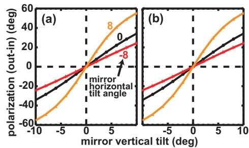
FIG. 7. (Color) Ray tracing calculation results for mirror tilting effect on the reflected polarization. The vertical axis is the difference between the incident and the reflected polarizations with the polarization of the incident light of (a)  $80^\circ$  and (b)  $105^\circ$ . The angle of incidence is  $15^\circ$  in both cases.
