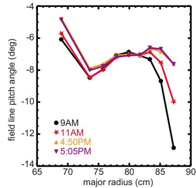
FIG. 3. (Color online) The tokamak pitch angle profiles from four beam-into-gas shots. All the shots have the same magnetic fields and gas pressure.
