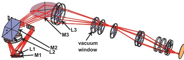
FIG. 1. (Color) Optical system layout of the MSE diagnostic in Alcator C-Mod. The small vertical rectangles are the footprints of the ten MSE channels along the diagnostic beam trajectory. A ray tracing example from the edgemoast channel is given. All the elements are enclosed by the stainless steel tubes (“canister”) which are not shown in the figure.
