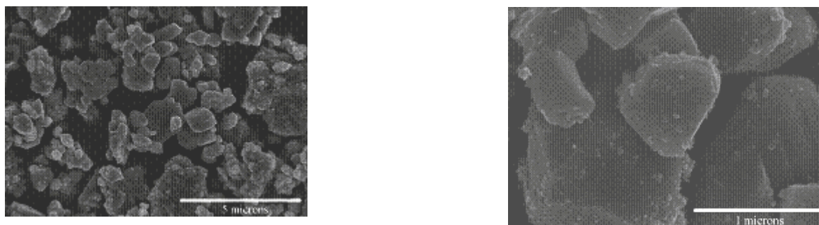
Figure 38. SEM micrographs of YEO powders coated with half amounts of \text{La}_{0.99}\text{Pr}_{0.01}\text{PO}_4 particles compared to those shown in Fig. 37.
