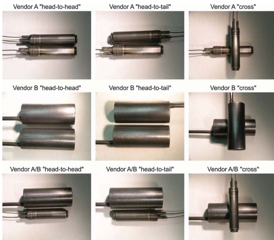
Figure 3-7. LVDT proximity configurations and combinations.
