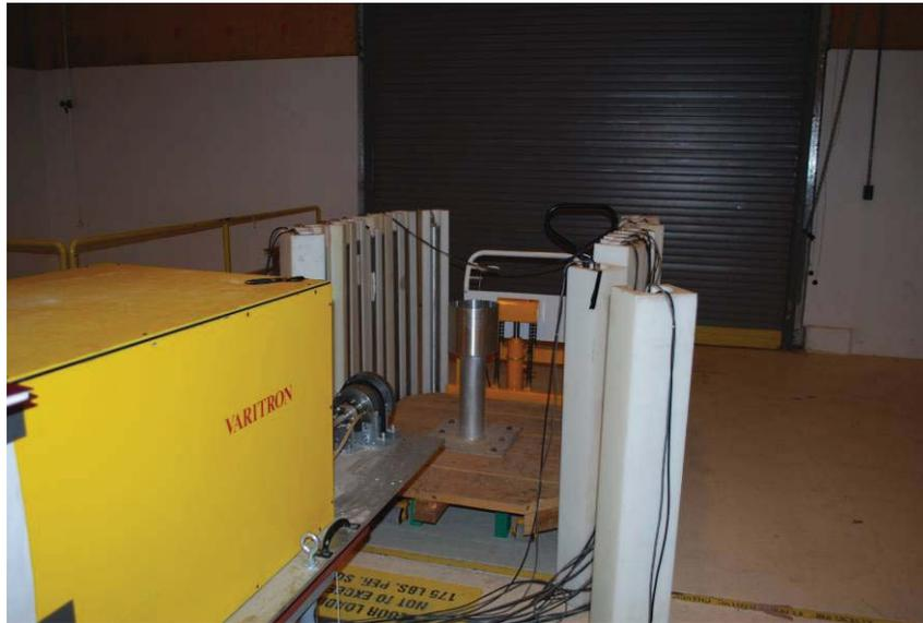
Figure 2-5. Experimental setup of the Varitron accelerator, the multiple PNDs positioned downstream of the accelerator, and the aluminum sample holder between two rows of PNDs.
