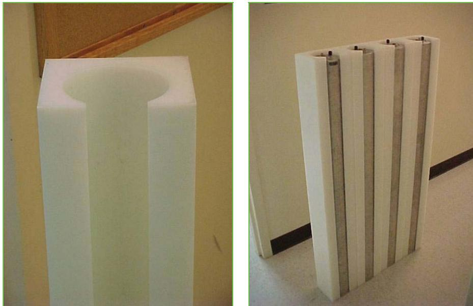
Figure 2-2. The PND cosmic background suppression shroud (left) and several PNDs with shrouds.
