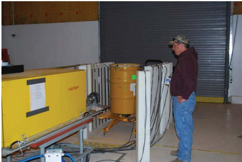
Figure 2-9. HEU-drum irradiation configuration. (Drum is centered on beam axis and its nearest surface is 1 m from photon source.)
