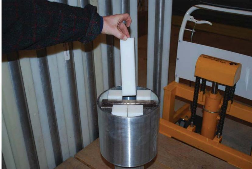
Figure 2-8. The selected polyethylene and bismuth composite shield configuration. (Nuclear material is sandwiched between slabs of 2.5 cm-thick bismuth and segments of 5.1 cm-square polyethylene.)
