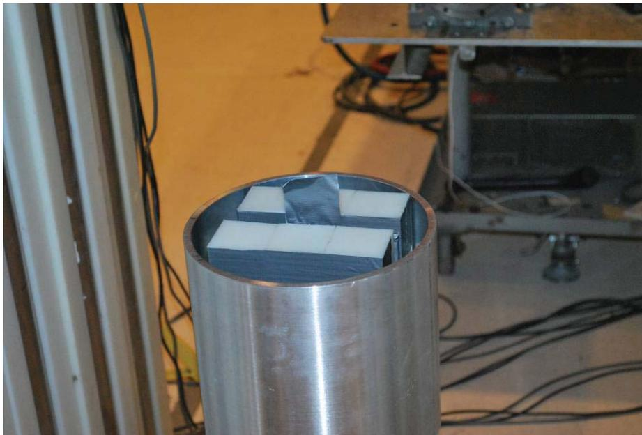
Figure 2-17. A typical shield configuration with the nuclear material positioned at 1.1-m from the photon source.
