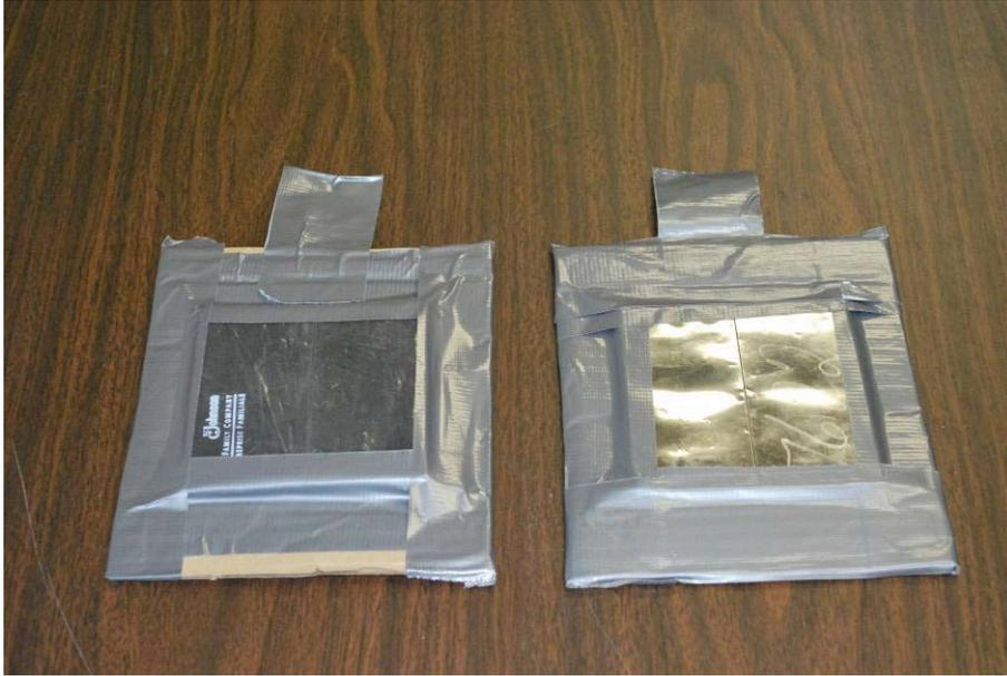
Figure 2-16. DU (left) and HEU (with stainless-steel cladding) used in FY-09 assessments.
