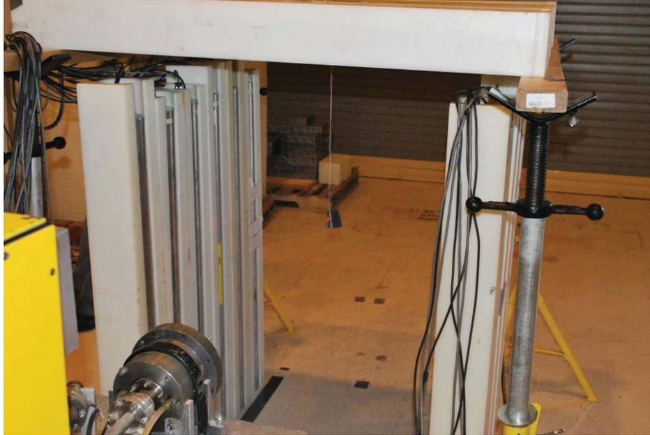
Figure 2-13. Calibration testing with the  $^{252}\text{Cf}$  sources. (Note the 1 m red alignment lasers on the source.)
