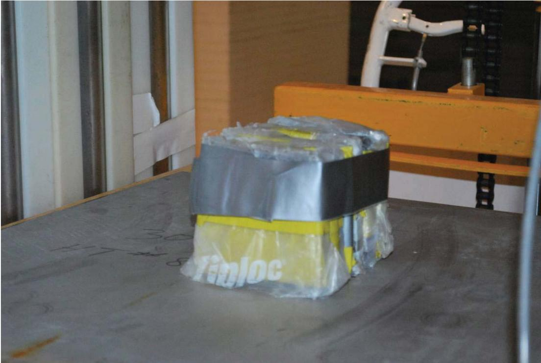
Figure 2-25. Maximum DU shield thickness for the two HEU plates (at nominal 1-m inspection position). The interrogating beam is incident normally on the DU with the accelerator to the left of the observer's position. For each thickness, DU is similarly configured on the front and back.
