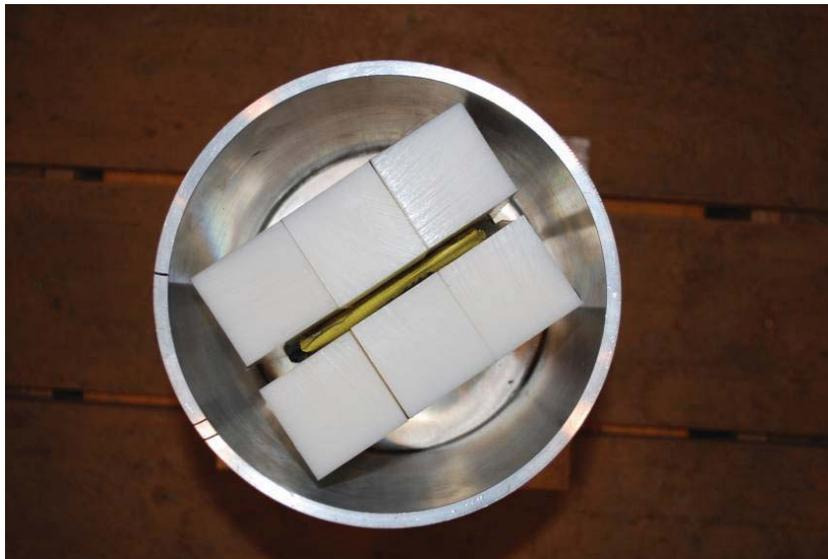
Figure 2-7. Polyethylene moderator sandwich configuration around DU.
