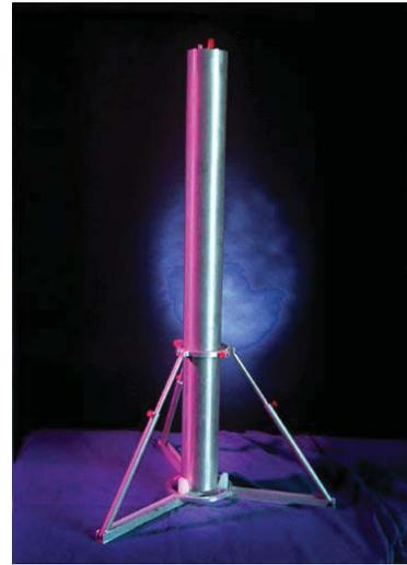
Figure 2-1. The Photonuclear Neutron Detector (PND).
