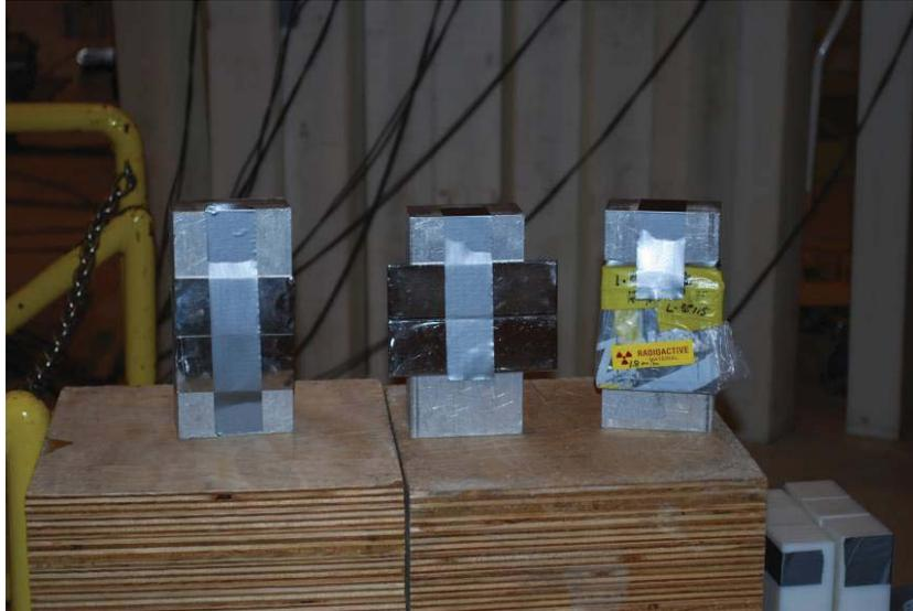
Figure 2-6. HEU, stainless-steel, and DU targets (left to right). (Note, aluminum bricks were used to align the targets with the beam axis when no additional moderator material was added.)
