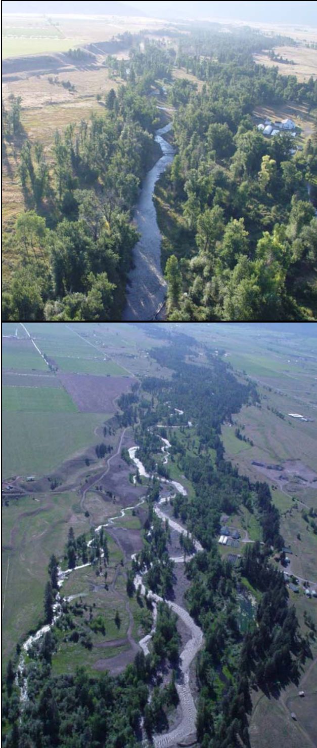
Figure 4. Aerial photo of the Jocko River through the Demonstration Reach Phase II project area prior to channel re-construction (left) and after channel reconstruction (right). In the post-construction photo, secondary channels are visible in the floodplain.
