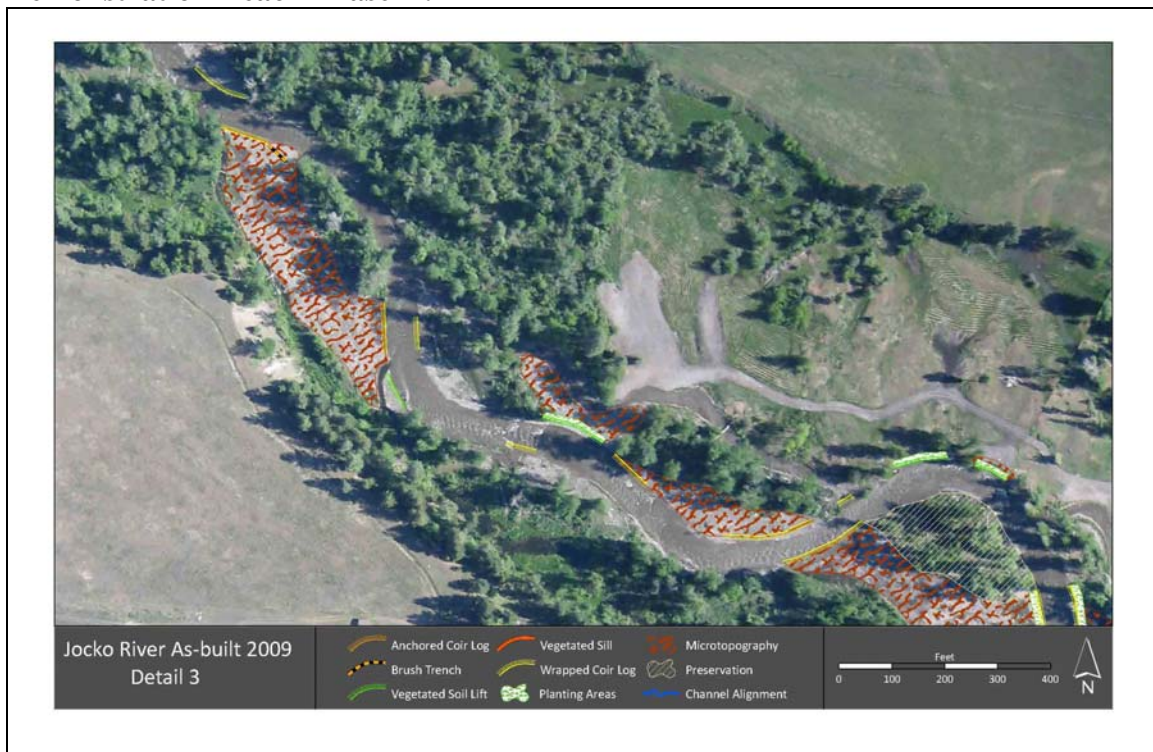
Figure 18. Detail figure of as-built conditions at the downstream section of the Demonstration Reach Phase II.
