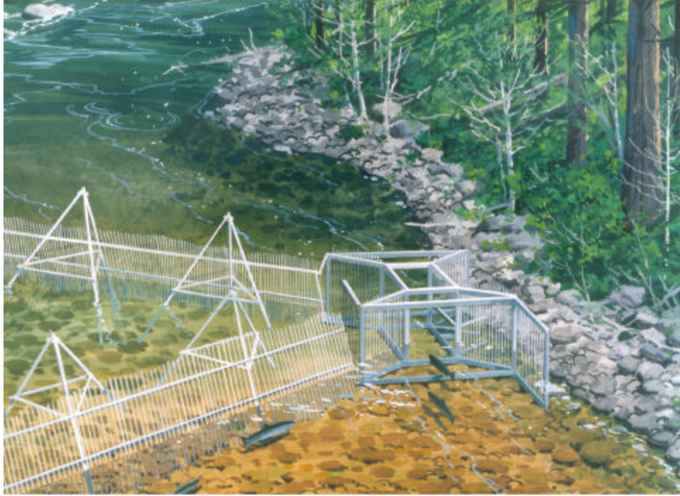
Figure 2. Artist's rendition of the underwater video fish counting station demonstrating the 0.9 by 0.7 m fish passage opening.
