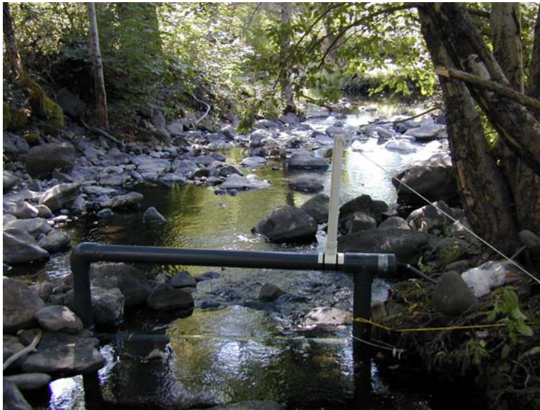
Figure 32. Photo of a pass-through PIT-tag antenna installed into Rattlesnake Creek. Note the stanchion mounted at the top of the antenna that is designed to break when heavy debris hits the antenna and the salvage line designed to help retrieve the loose antenna.
