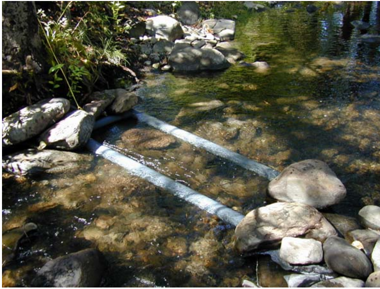
Figure 31. Photo of a pass-by antenna installed into Rattlesnake Creek.
