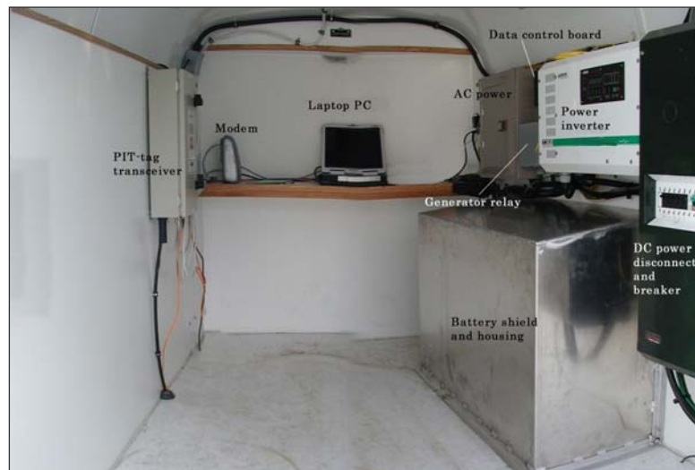
Figure 34. Outside and inside views of the PIT-tag equipment trailer that show the equipment for power management and communications.
