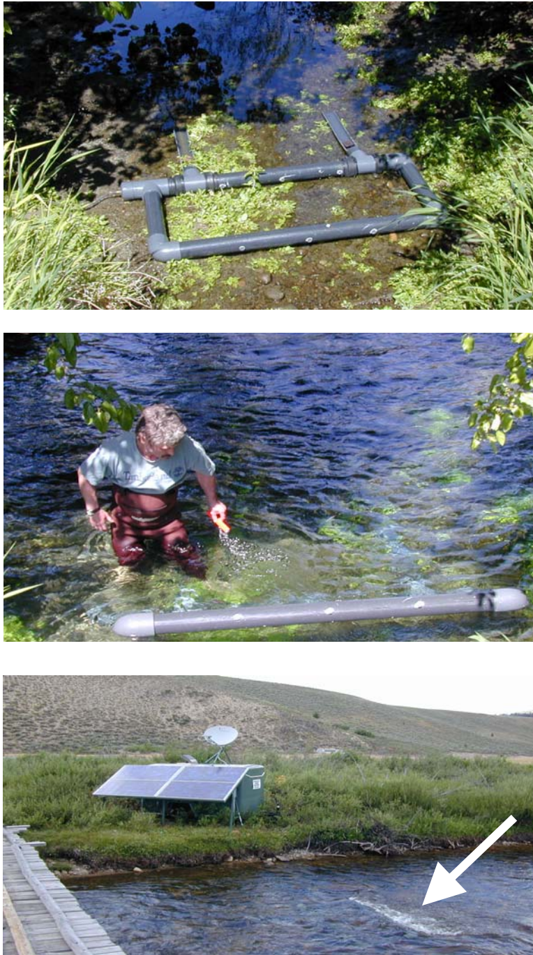
Figure 33. The hybrid PIT-tag antenna under low (top), medium (middle), and high (bottom) water conditions. Low and medium water photos were taken while the antenna was being developed in a stream near Pasco, WA; high water photo shows the antenna operating in Valley Creek, ID.
