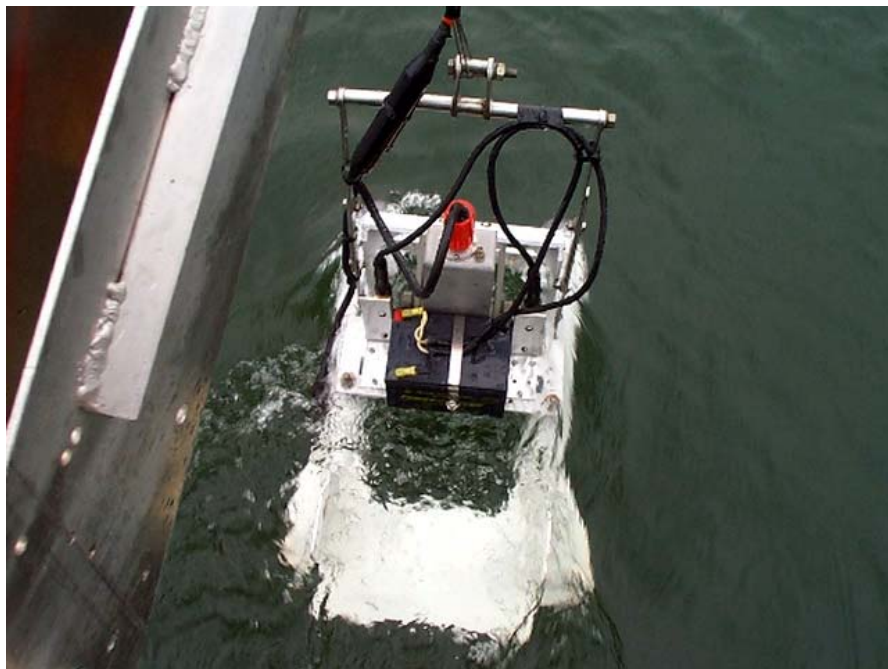
Figure 3. Photo of weighted sled with video camera and lasers used to collect substrate images
