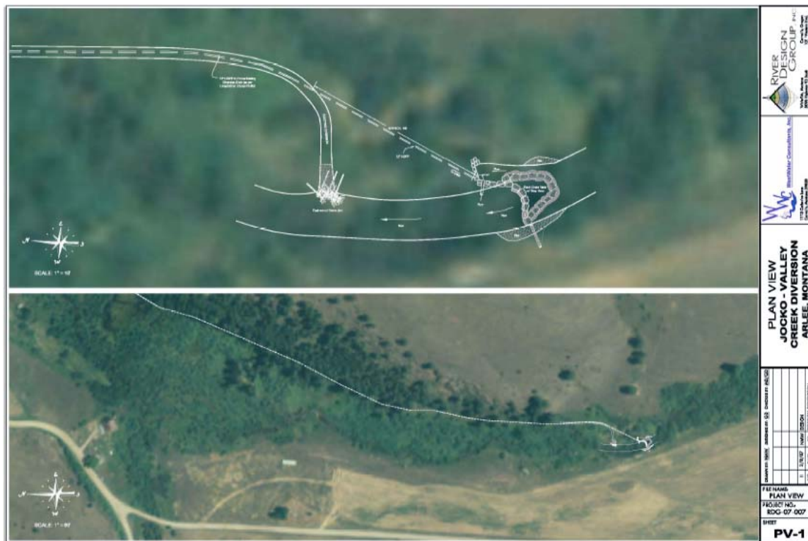
Figure 18: Plan view of the Morin ditch pipeline diversion structure.
