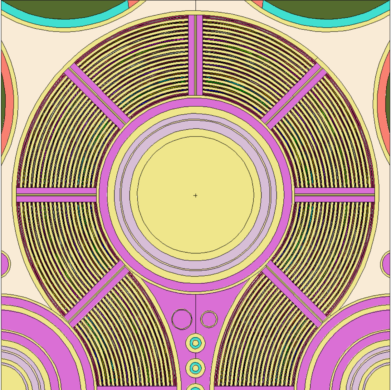
Figure 2.4: Northwest Flux Trap containing a Water-Filled Pressure Tube and Insulation Tube.
