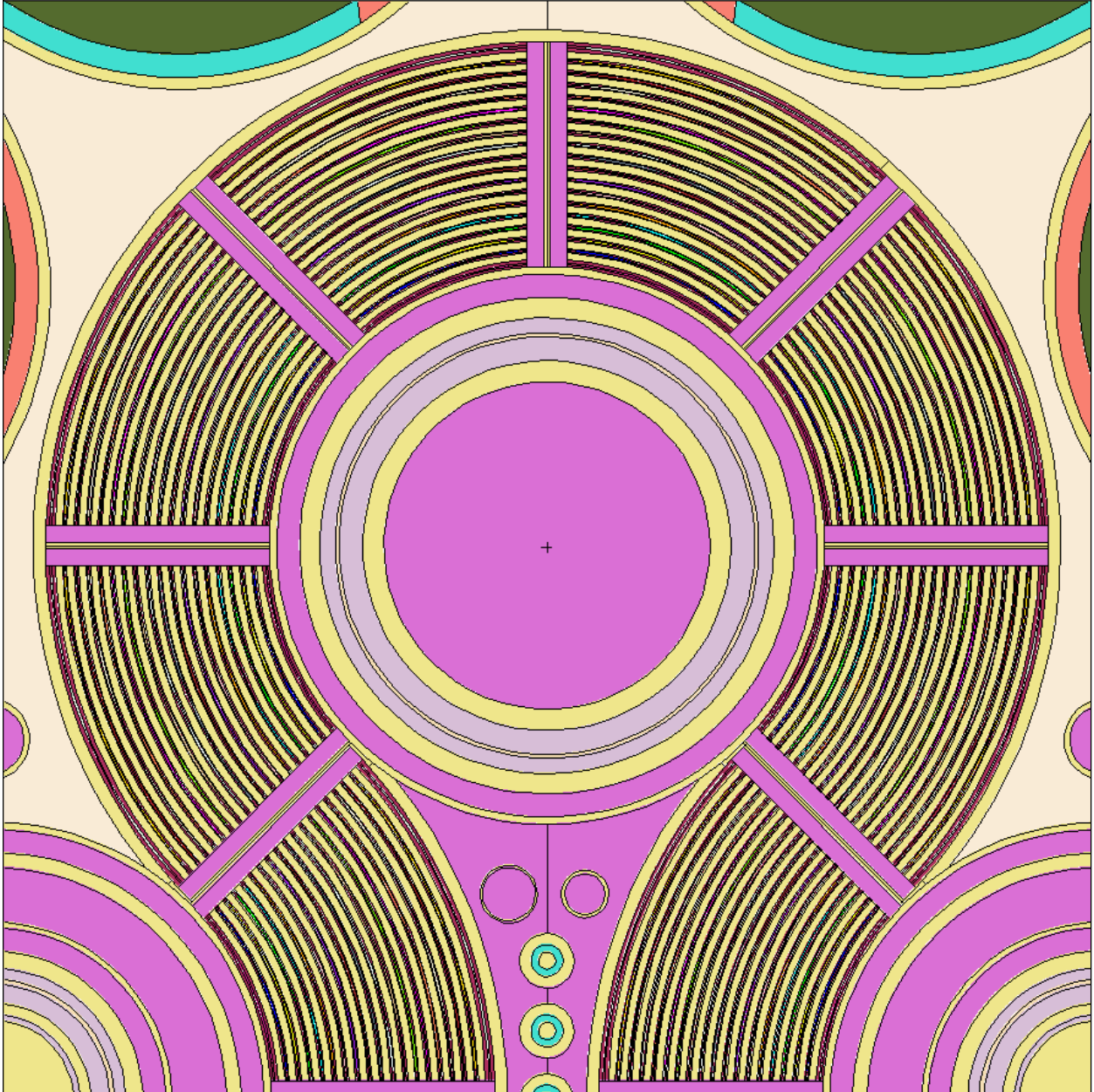
Figure 2.3: Northwest Flux Trap (Benchmark Model) containing an Aluminum Filler, Pressure Tube, and Insulation Tube.
