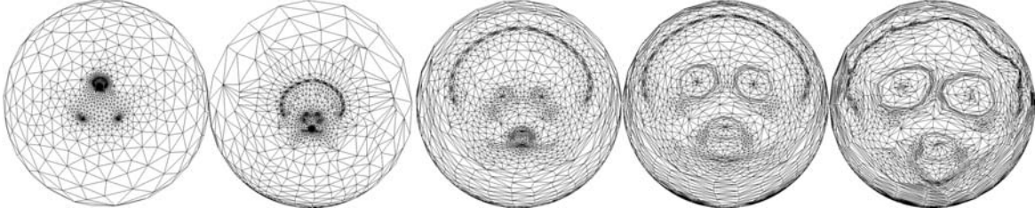
Figure 6: Results of spherical parameterization of a triceratops model using various schemes (leftmost: simplest, Tutte-like embedding) that preserve either angles (2 nd from left) or areas (last), or even linear combinations of them (middle ones).
