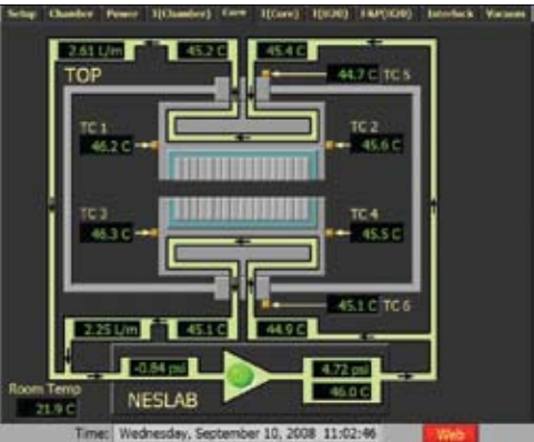
The X9 mini-gap undulator bakeout monitor
