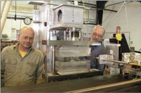
Michael Lehecka (left) and George Rakowsky setting up the X9 MGU for Hall probe field mapping in the Magnetic Measurement Lab.
