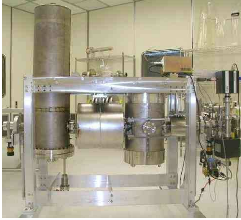
Figure 15. Cold mass assembly on titanium alignment rails inside the clean room. From left: QWR with RF coupler, solenoid with Nb shield, HWR with upper and lower cryoperm shield pieces, and quadrupole.
