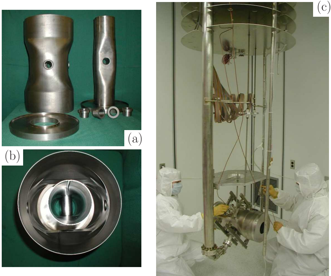
Figure 2. (a) Niobium parts before final welding of HWR prototype; (b) inside view of the cavity before assembly of upper plate; (c) assembly of the cavity onto the insert for cryogenic testing.
