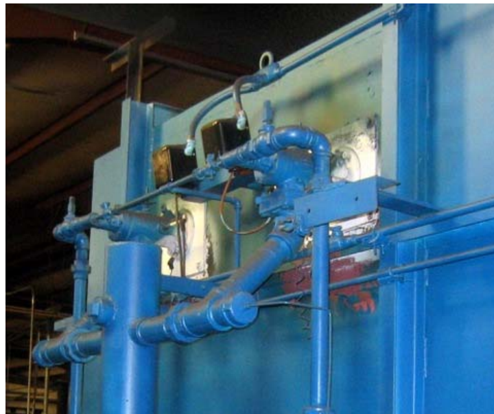
Figure 2. View of Eclipse burners installed in heat treating furnace.
