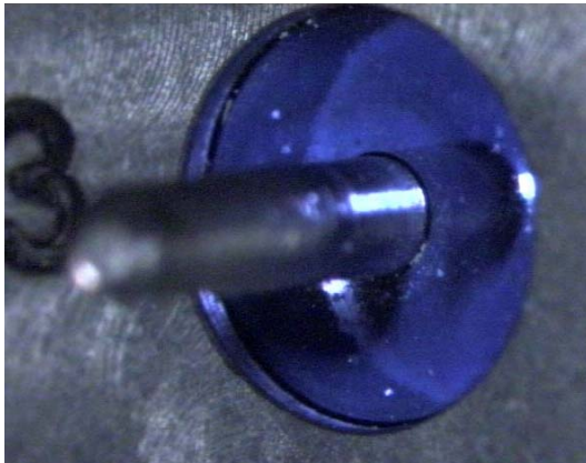
Figure 32. Test pin and sealing glass after solder and thermal cycling tests.
