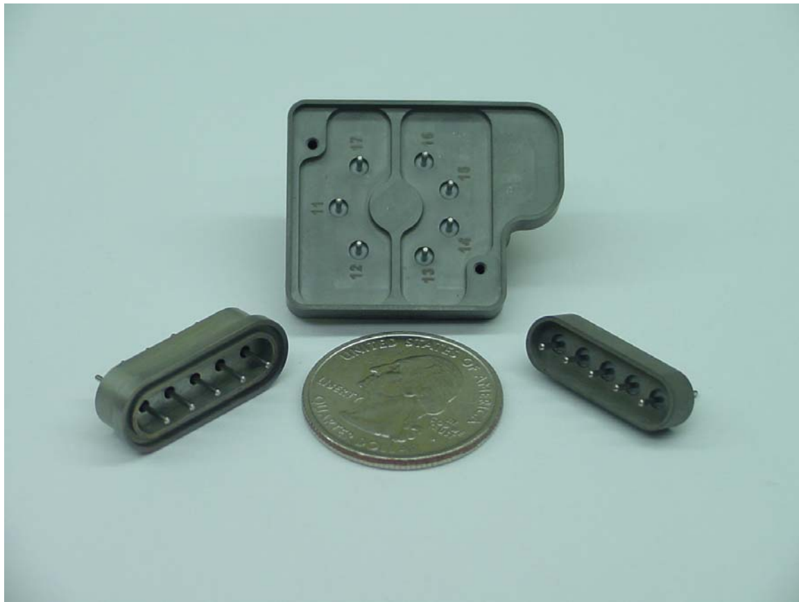
Figure 9. Photographs of glass-to-metal seal headers. Bottom left: Input header assembly (combines header and web which was previously a welded assembly, thus eliminating a weld process). Center: Utility header. Bottom right: Output header
