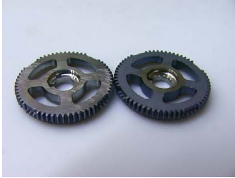
Figure 15. ISL shutter gear; no lubrication (left) and with lubrication (right)
