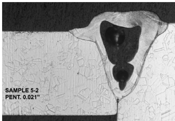
Figure 22. Weld porosity (gas pockets) from coating contamination
