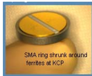
Figure 24. SMA Captured Ferrites
