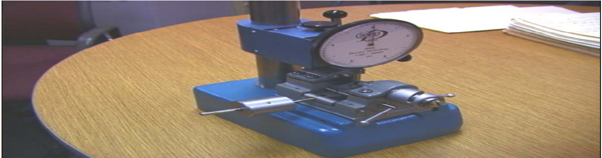
Figure 21. Bearing Push & Radial Fixture
