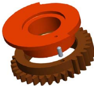
Figure 10. Mistake Proofing Pin Added
