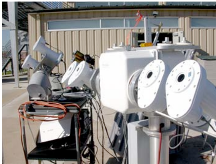
Absolute Cavity Radiometers on Solar Trackers
