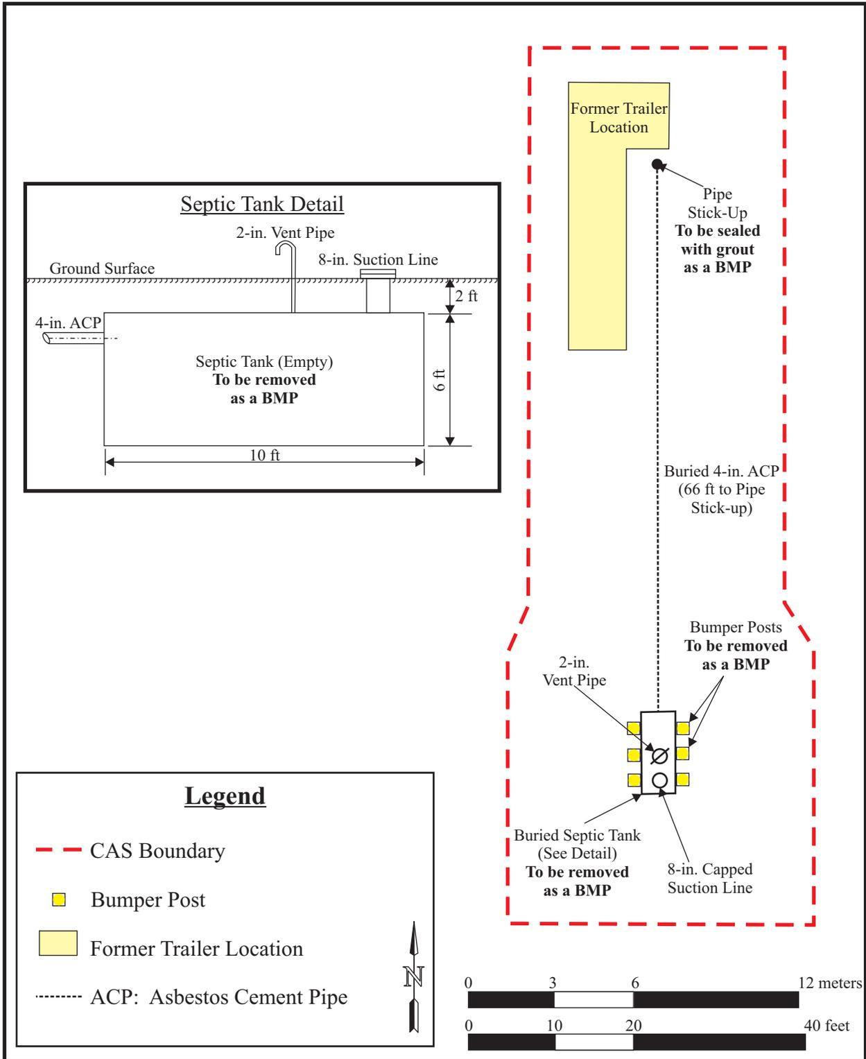
**FIGURE 2. CORRECTIVE ACTION SITE 03-04-02, AREA 3 SUBDOCK SEPTIC TANK**
