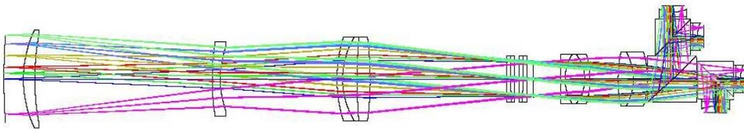
Figure 1. Design of simultaneous four-band imaging system, using a triplet of cube beamsplitters. The cube triplet splits the beam into four distinct optical passbands, each of which is imaged on a focal plane array.
