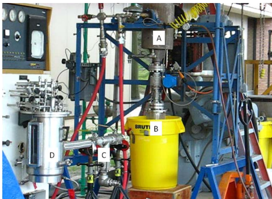
Figure 29. Pilot Plant Equipment Set-Up. (A) Reactor used during biomass pretreatment and separate hydrolysis and fermentation (SHF); (B) Double-walled stainless steel cylinder attached to the bottom of the reactor post pretreatment for the washing and removal of inhibitors (optional), (C) Flexible stainless steel hose fitted to a T valve for the transfer of partially liquefied biomass to a 30 L bioreactor post SHF, (D) Bioreactor where liquefied biomass was collected in batches for the production of ethanol during simultaneous saccharification and fermentation (SSF).
