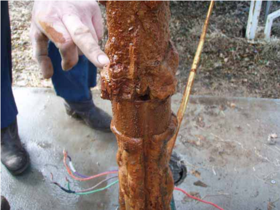
FIGURE 3.2 Corrosion and perforation identified in the steel riser pipe of well GWEX1, March 2008.
