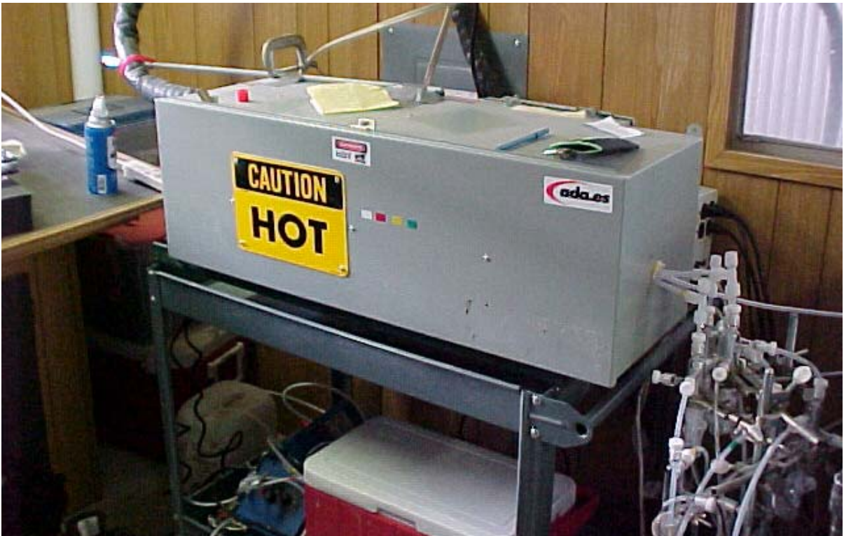
Figure 5. Sorbent Screening Device—Heated Box and Impingers.
