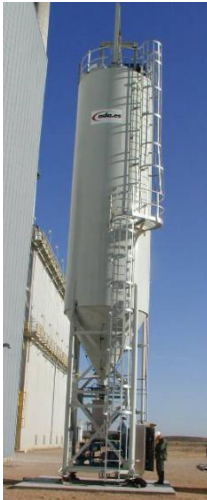
Figure 1. Carbon Injection Storage Silo and Feeder Trains for 150 MWe (Phase I System).
