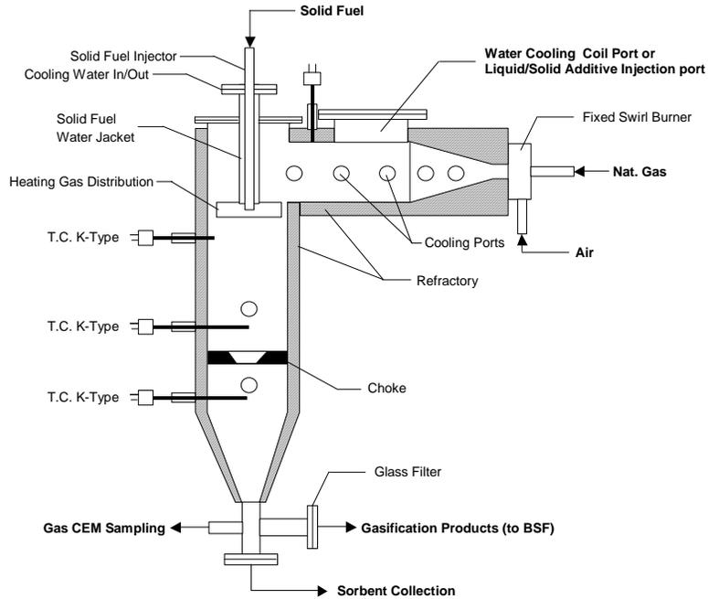
**Figure 3-1. Schematic of Pilot-Scale Gasifier.**
