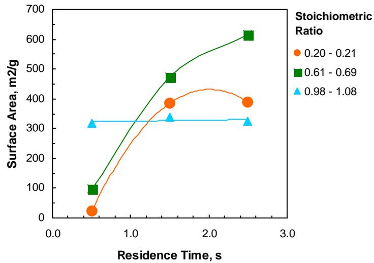
**Figure 4-7. Impact of residence time on subbituminous coal sorbent surface area.**
