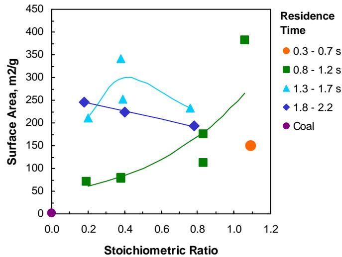
**Figure 4-3. Impact of stoichiometric ratio on Bituminous Coal #2 sorbent surface area.**
