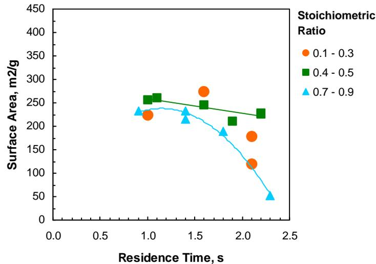
**Figure 4-2. Impact of residence time on Bituminous Coal #1 sorbent surface area.**
