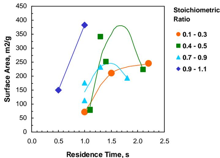
**Figure 4-4. Impact of residence time on Bituminous Coal #2 sorbent surface area.**
