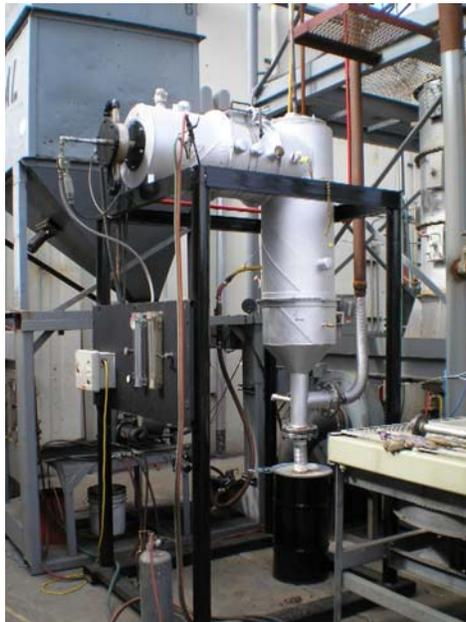
**Figure 3-2. Photograph of Pilot-Scale Gasifier.**
