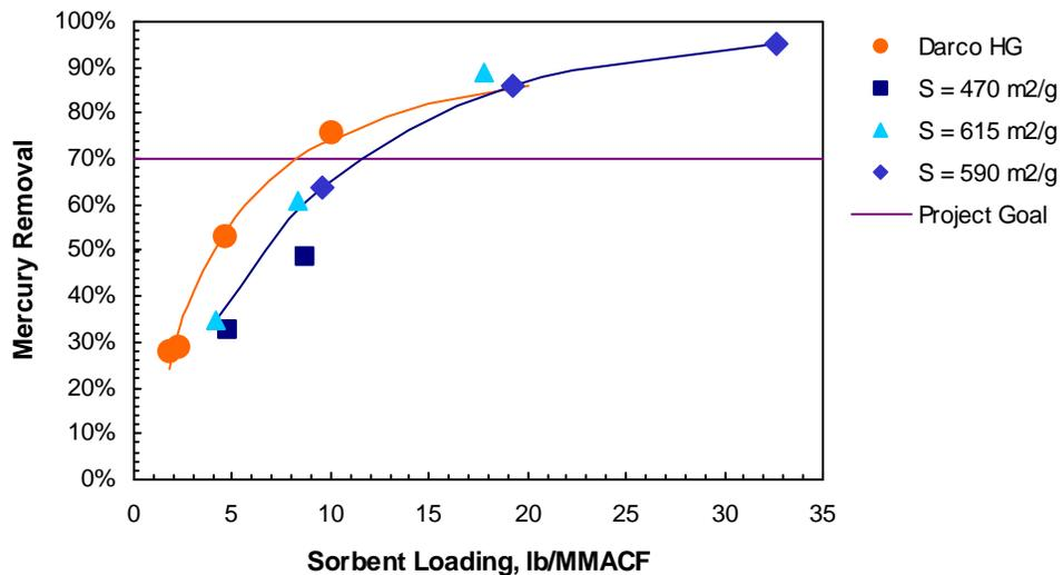
Figure 5-1. Gasification-generated sorbent mercury removals.
