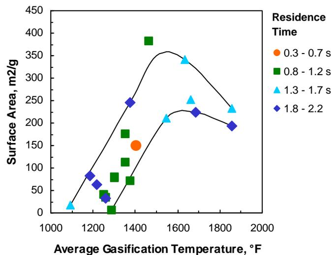
Figure 4-5. Impact of temperature on Bituminous Coal #2 sorbent surface area.
