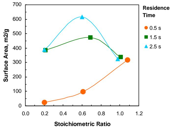
**Figure 4-6. Impact of stoichiometric ratio on subbituminous coal sorbent surface area.**
