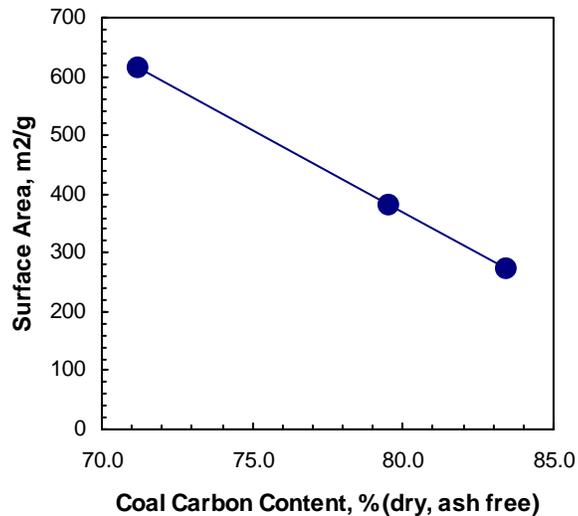
**Figure 4-8. Impact of coal carbon content on maximum sorbent surface area.**
