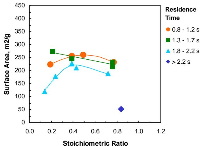
Figure 4-1. Impact of stoichiometric ratio on Bituminous Coal #1 sorbent surface area.
