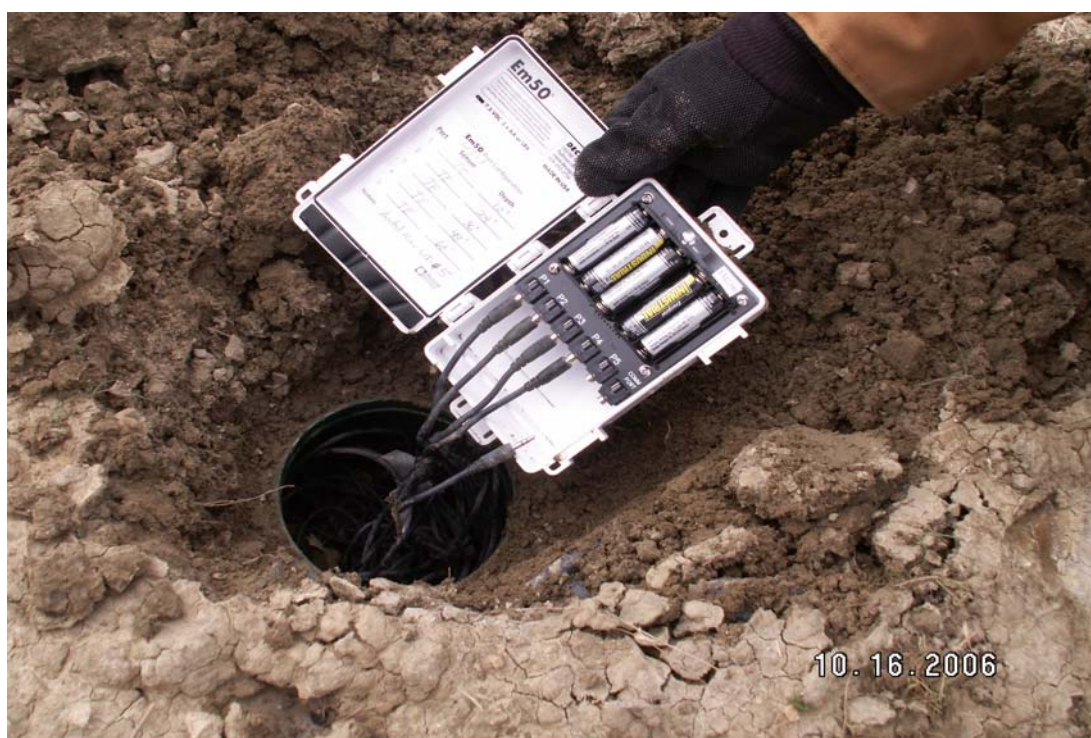
Figure 7.7: Em50 Decagon data logger with underground connections to soil probes measuring soil water content, soil EC and soil temperature.
