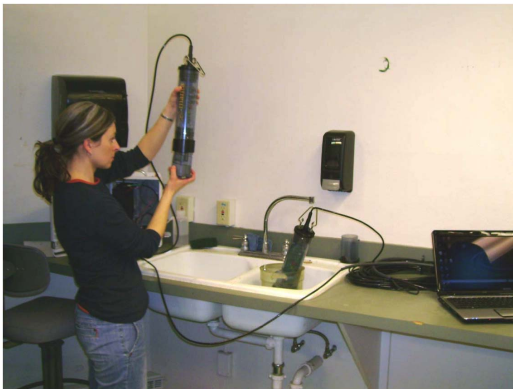
Figure 11.9: Office testing of water quality multiprobe.
