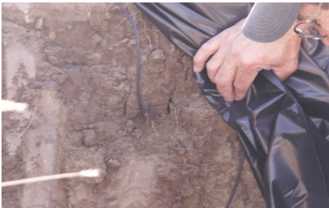
Figure 7.6: Installation of the ECH 2 O soil probes measuring soil water content, soil EC and soil temperature.
