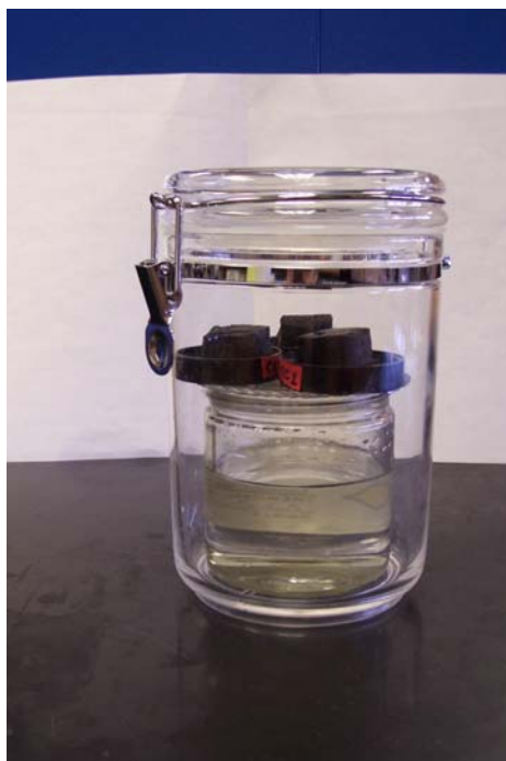
Figure 2.1: Experimental Setup for Water Adsorption Isotherms
