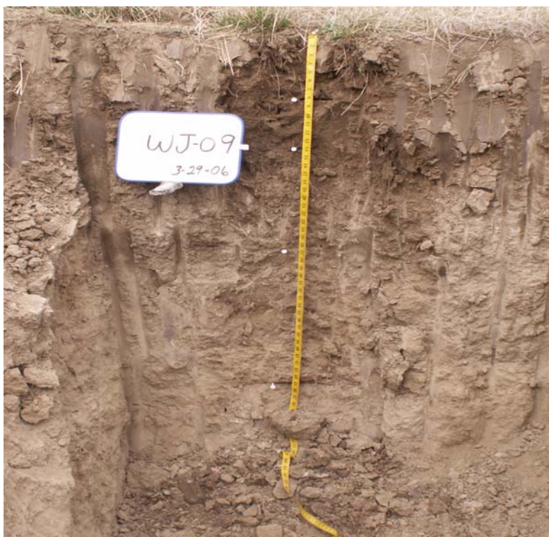
Figure 7.3: Typical soil profile associated with the WJ research site.
