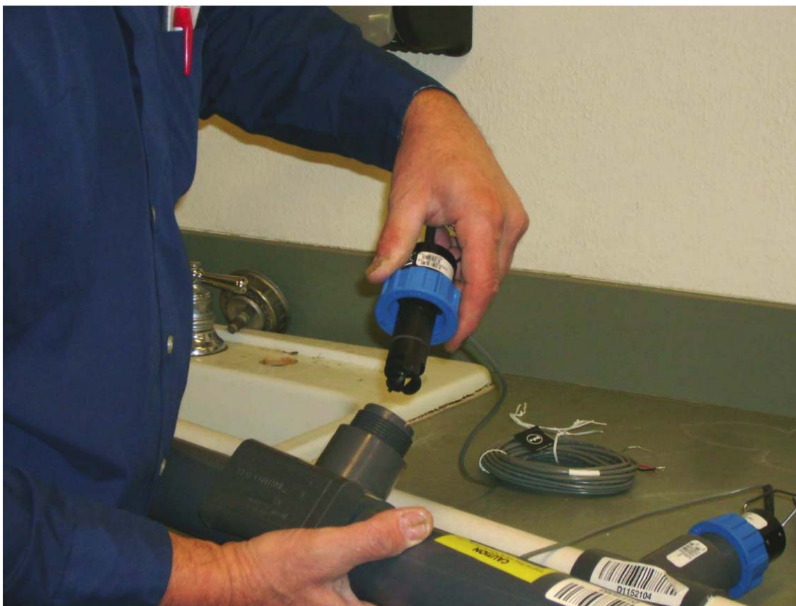
Figure 11.6: Assembly of flow meter.
