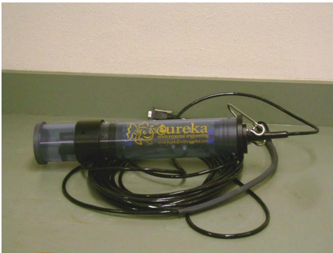
Figure 11.8: Water quality multiprobe.
