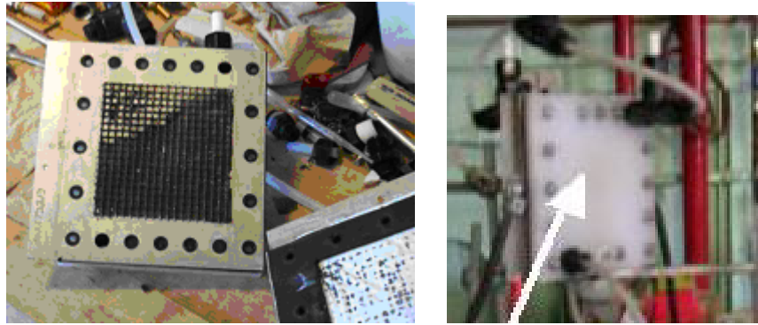
Figure 12: (a) Image of bench-scale experiment #3B showing coating effectiveness and (b) single-cell device illustrating orientation of flow passages.
