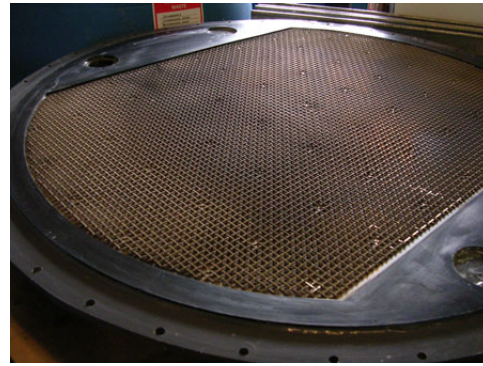
Figure 15: (a) Image showing well-adhered electrode coating after cleaning with nitric acid; (b) uniform coating of electrode surface for this experiment using the full-size deposition rig.
