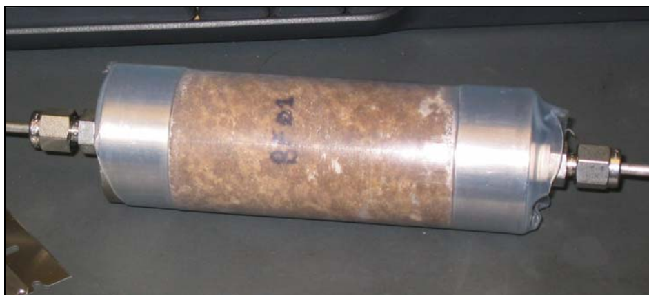
Plate 8 Core covered with Teflon® heat shrink material
