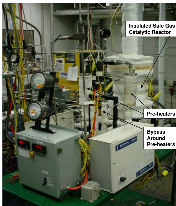
Figure 9. Intermediate-Scale Start Gas Test Hardware
