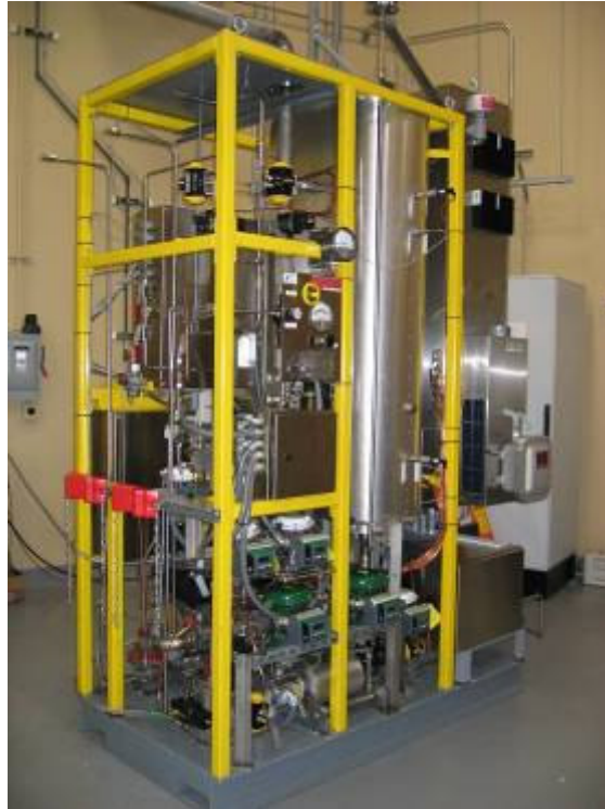
Figure 14. Skid with Desulfurizer Subsystem and CPOX controls
