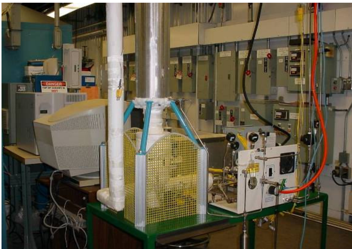
Figure 5. High-Pressure CPOX Test Stand
