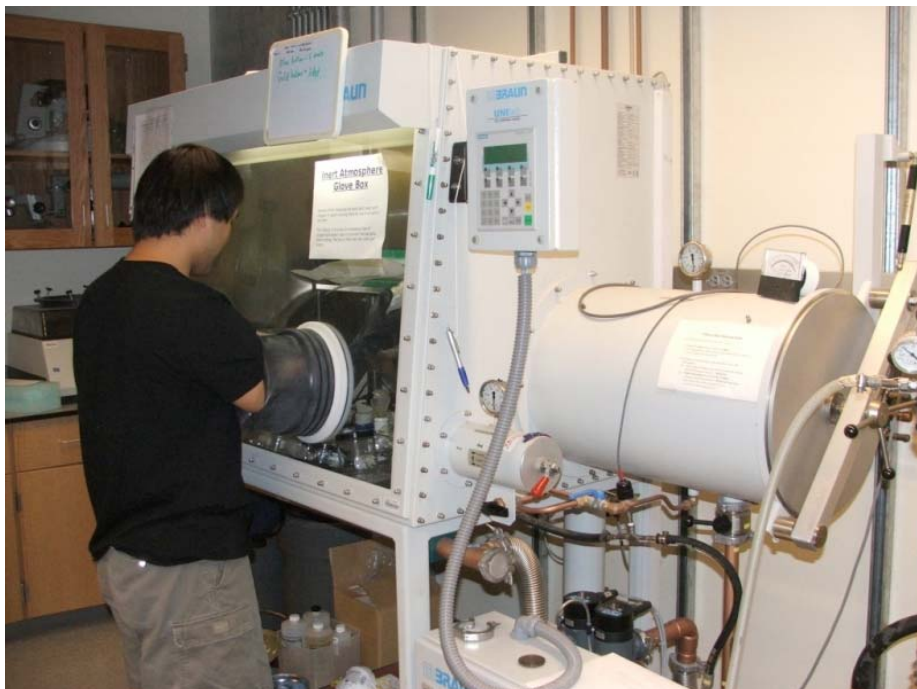
Figure 1.2 – The argon glove box serves to handle and store air sensitive materials.
