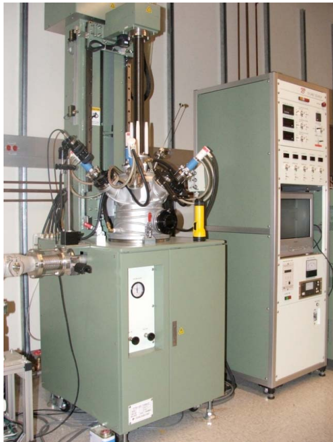
Figure 1.3 – The tetra-arc furnace in its current location. The CCD camera mounted outside of one of the three window ports allows us to record the growth in a video. Videos can be viewed at our website ( http://mbmlab.ucsd.edu/facility.html ).
