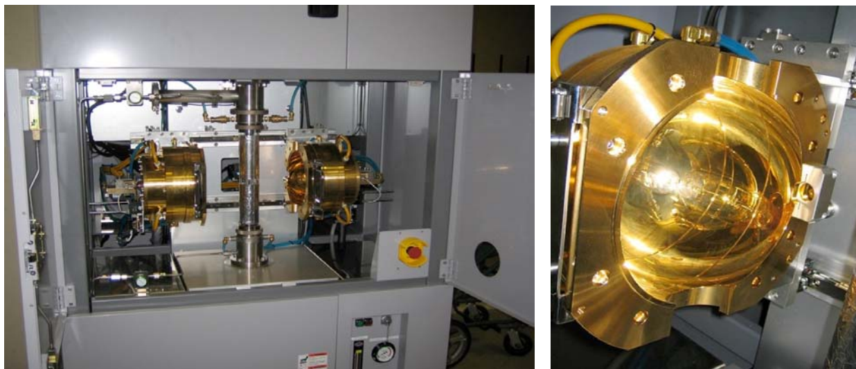
Figure 1.5 – ( Left ) The image furnace main chamber. ( Right ) Detail of one of the gold-plated mirrors.
