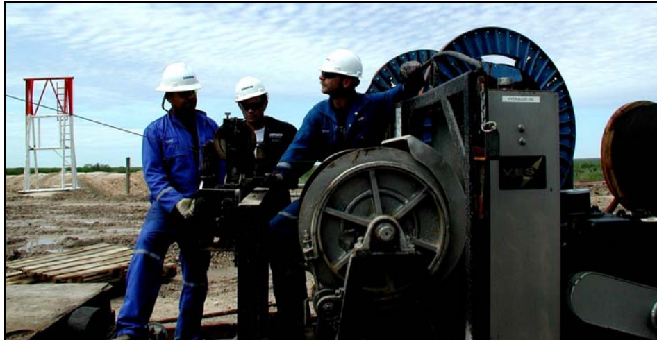
Figure 28. Retrieving the HPHT MWD tool via slickline.
