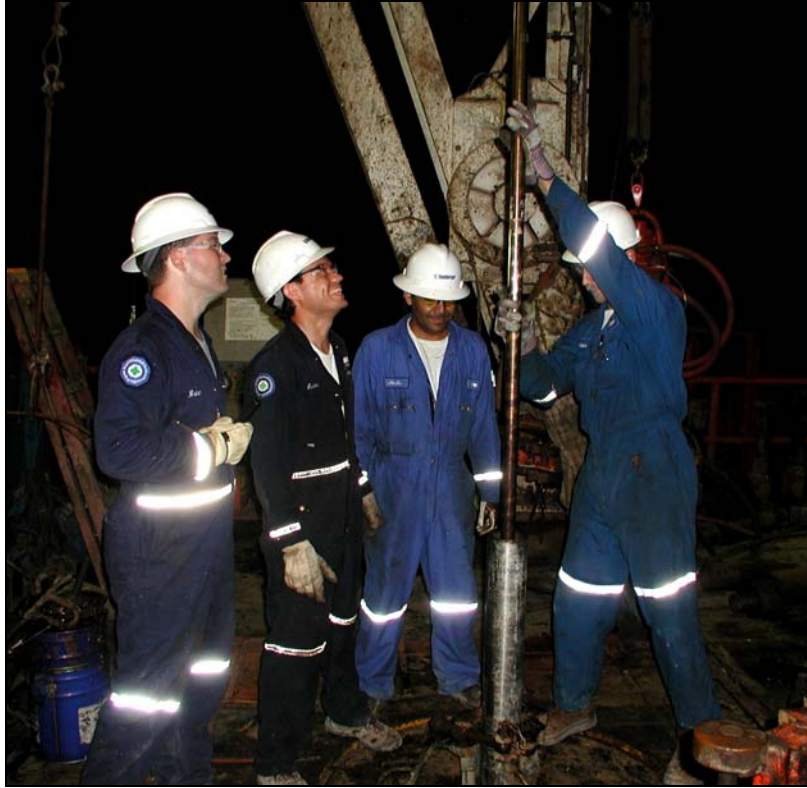
Figure 26. Installing the HPHT MWD tool in the NC38-47 collar.
