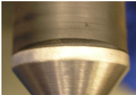
Figure 37. Inductive stinger tip damage.
