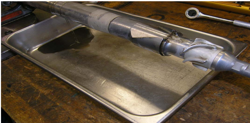
Figure 35. Primary compensator oil volume, mud invaded.
