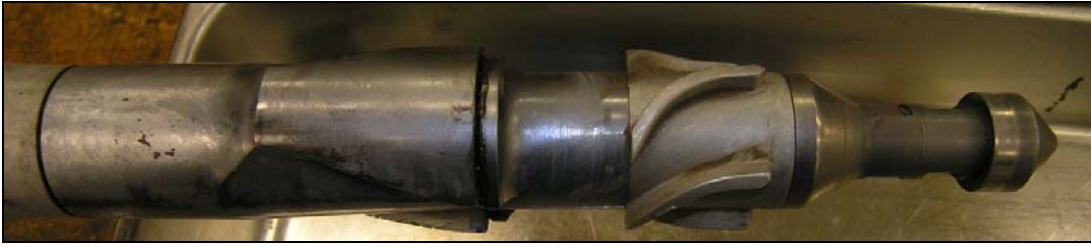
Figure 34. Separation Between Modulator Stator and Stator Adapter
