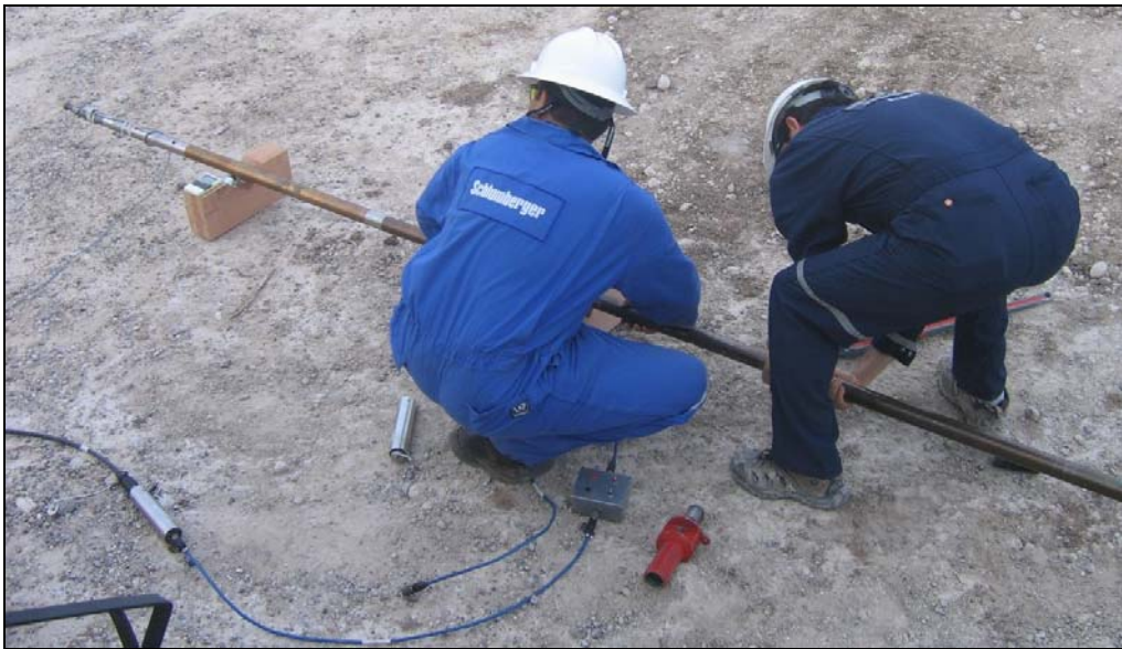
Figure 23. Surface testing the HPHT MWD tool.
