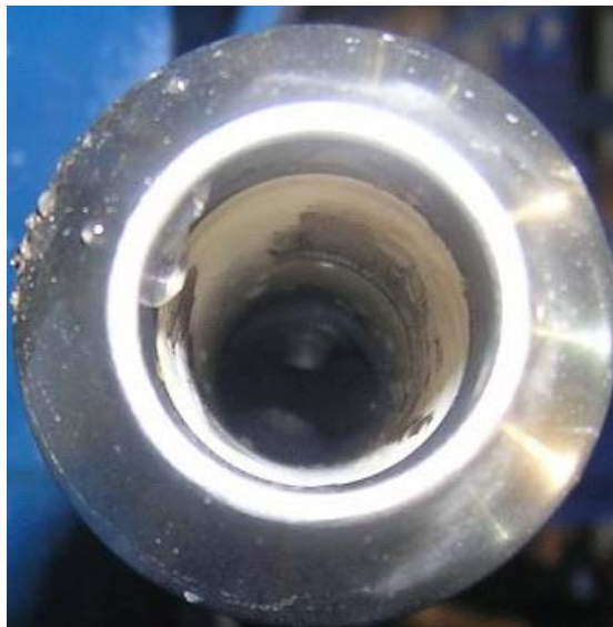
Figure 38. Inductive coil with internal mud buildup.
