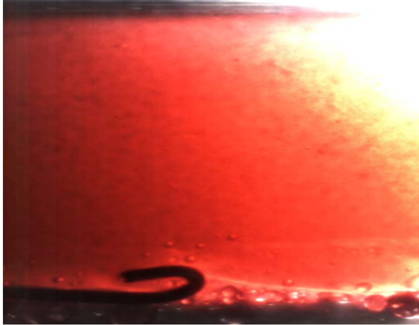
Figure 36 - v_{so}=0.500 m/s v_{sw}=0.025 m/s (DW/O&O)
