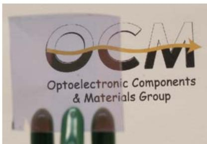
demonstrating the first semitransparent organic photovoltaic. The cathode consisted of a very thin (~10 nm) Ag layer, followed by a thicker layer of ITO. Cell efficiencies were not degraded from their values using a metal contact, provided that the optical absorption through only a single pass of the light through the device (as opposed to the reflective, double pass of thick metallic cathodes) was taken into account. These devices have
