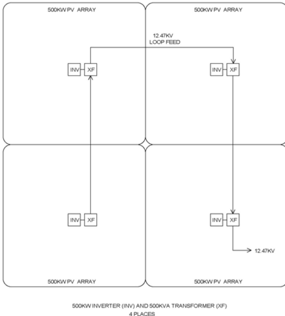
**Figure 8 - Solution #1 Field Layout, 4 x 500KVA Transformers**
