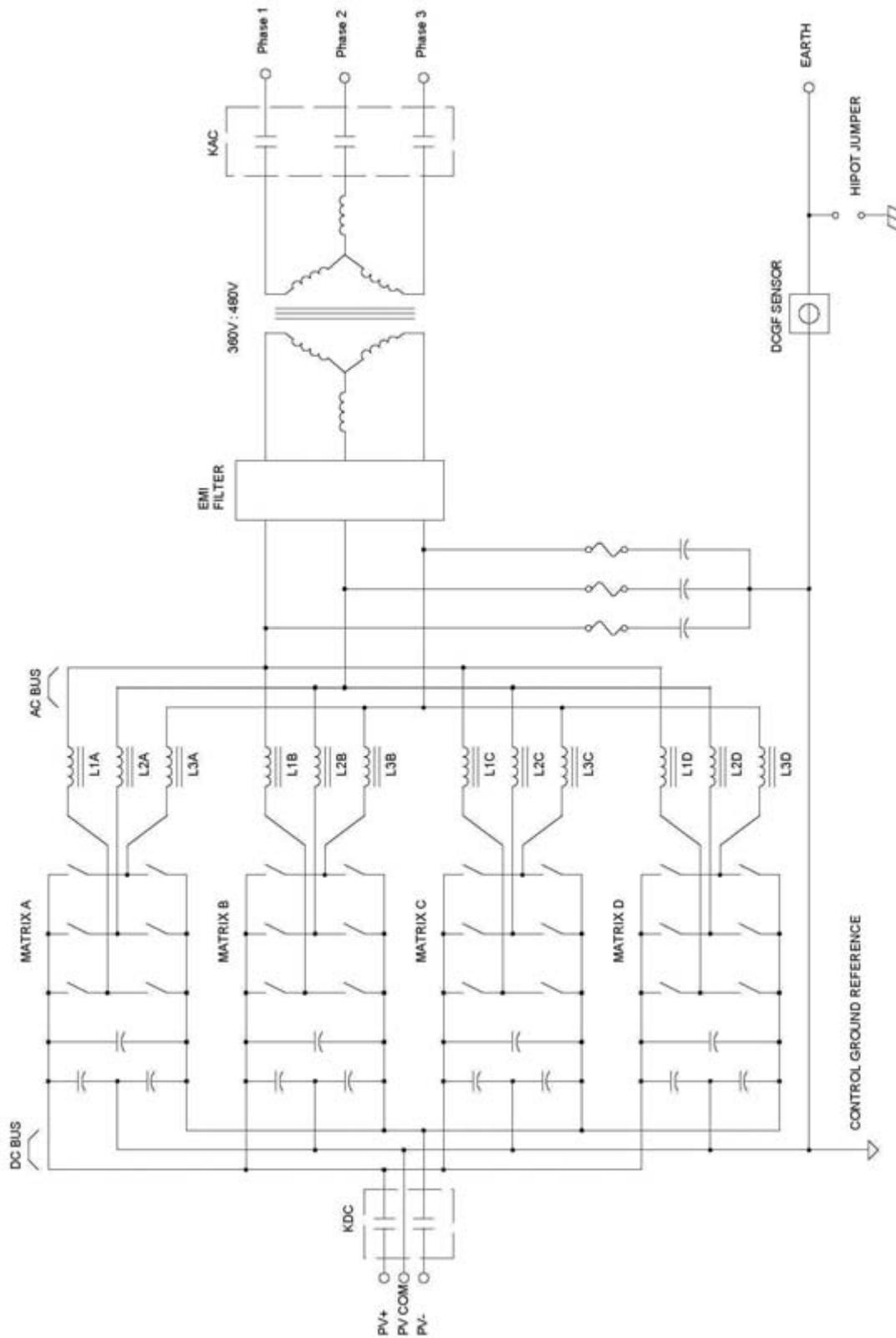
Figure 2 - Inverter Power Architecture
