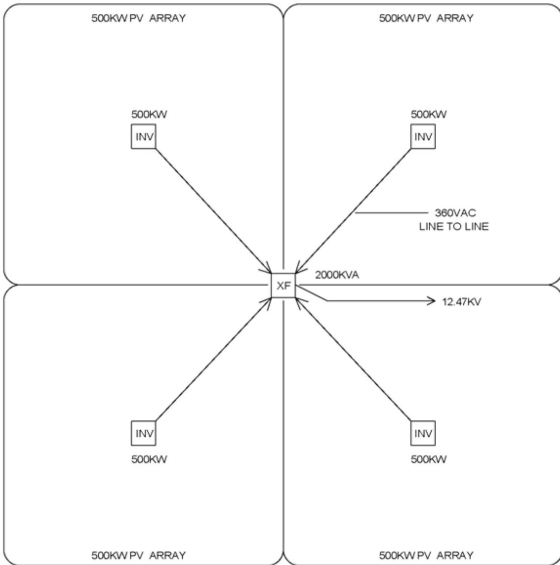
**Figure 10 - Solution #2 Field Layout, 2MVA Transformer**
