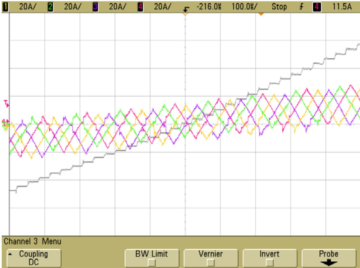
**Figure 19 - Interleaved High Frequency PWM Switching**
