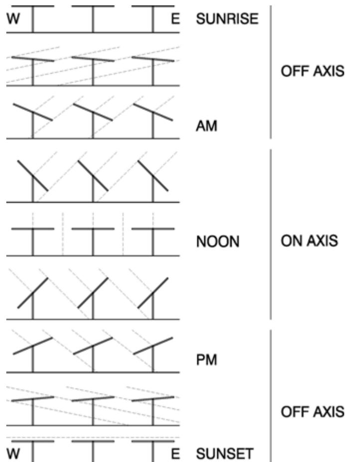
Figure 15 - Tracker Controller Software Anti-Shadowing Algorithm
