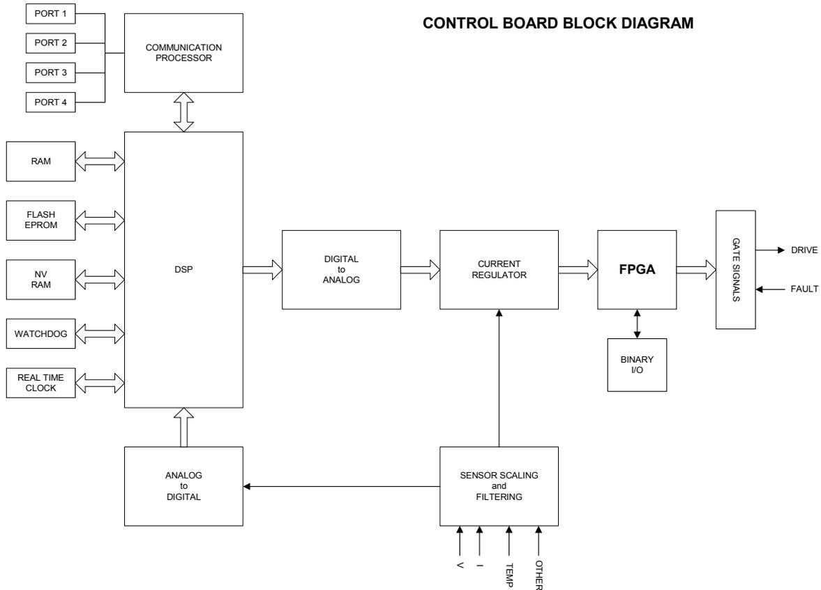
**Figure 6 - DSP Control Board Block Diagram**
