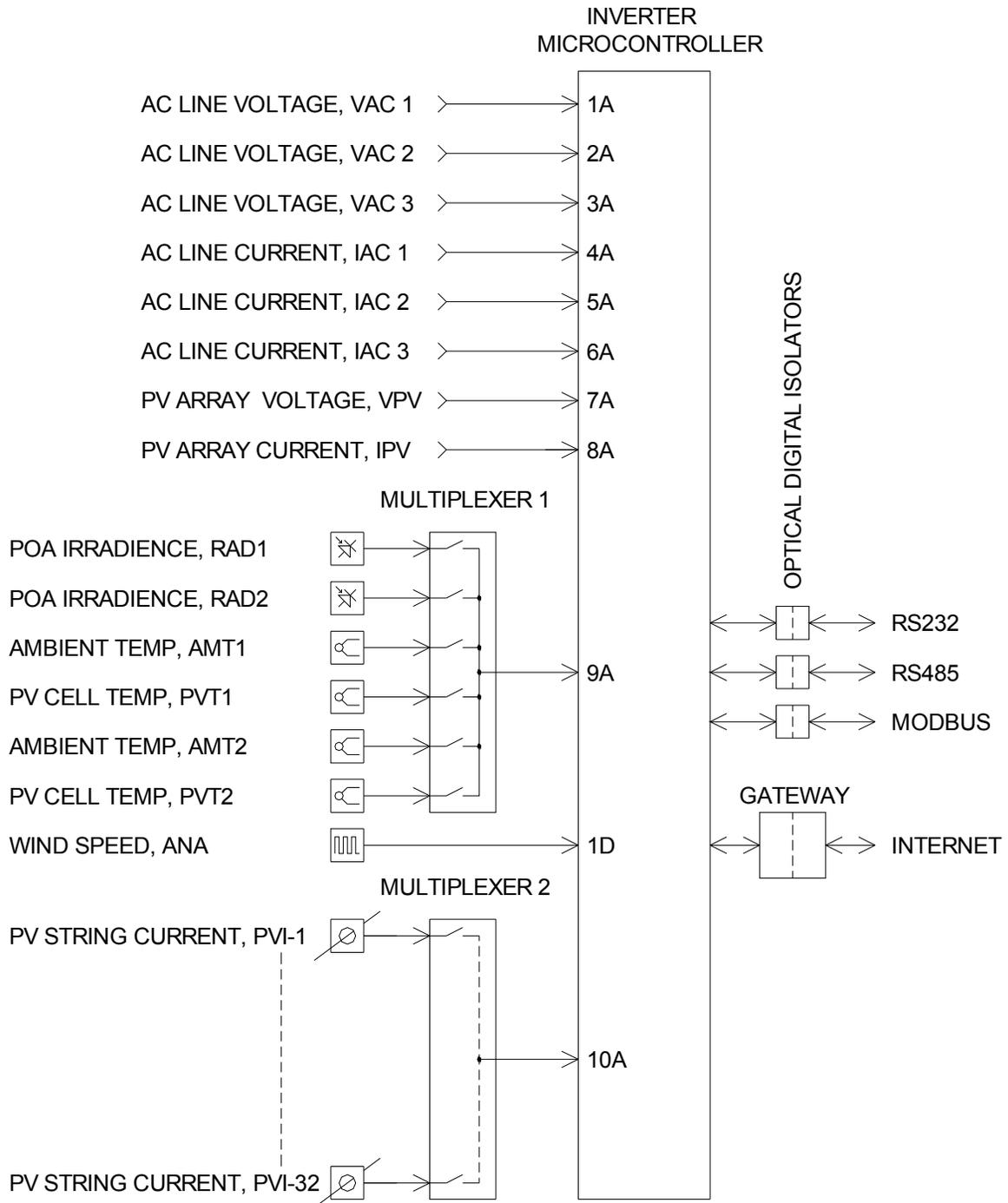
**Figure 12 - System Integrated Communications Design Block Diagram**
