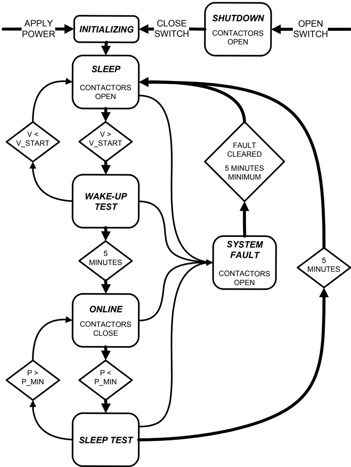
Figure 13 - State Machine Diagram
