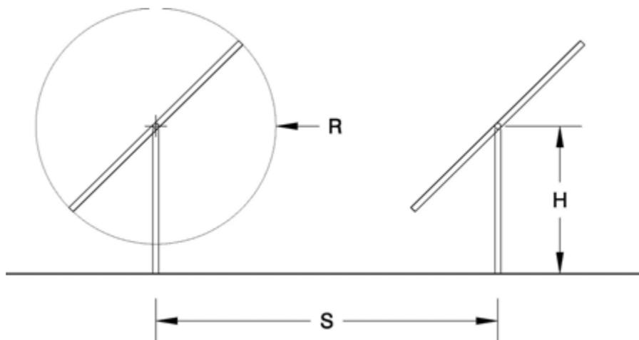
**Figure 16 – Programmable Array Form Factor Parameters**
