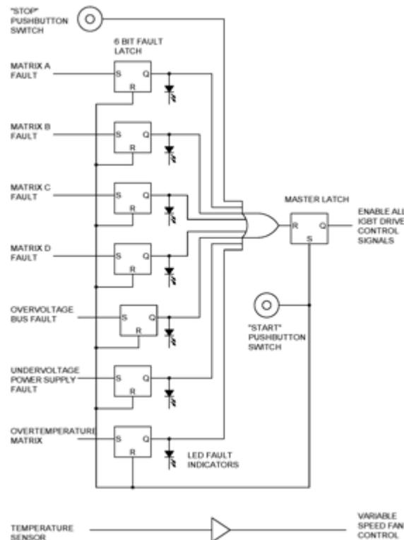
**Figure 5 - Analog Control Board Fault Detection**
