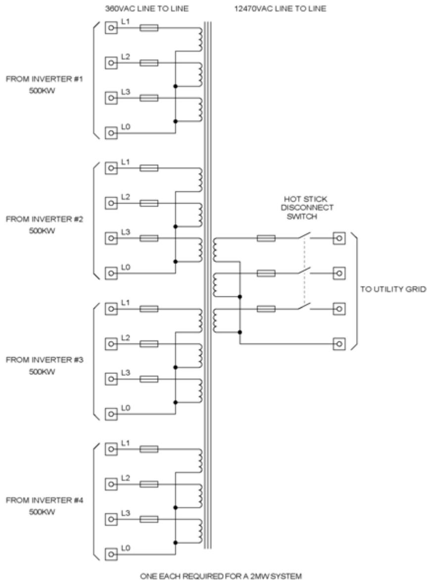
**Figure 11 - Solution #3, 2MVA Transformer Subassembly Schematic**
