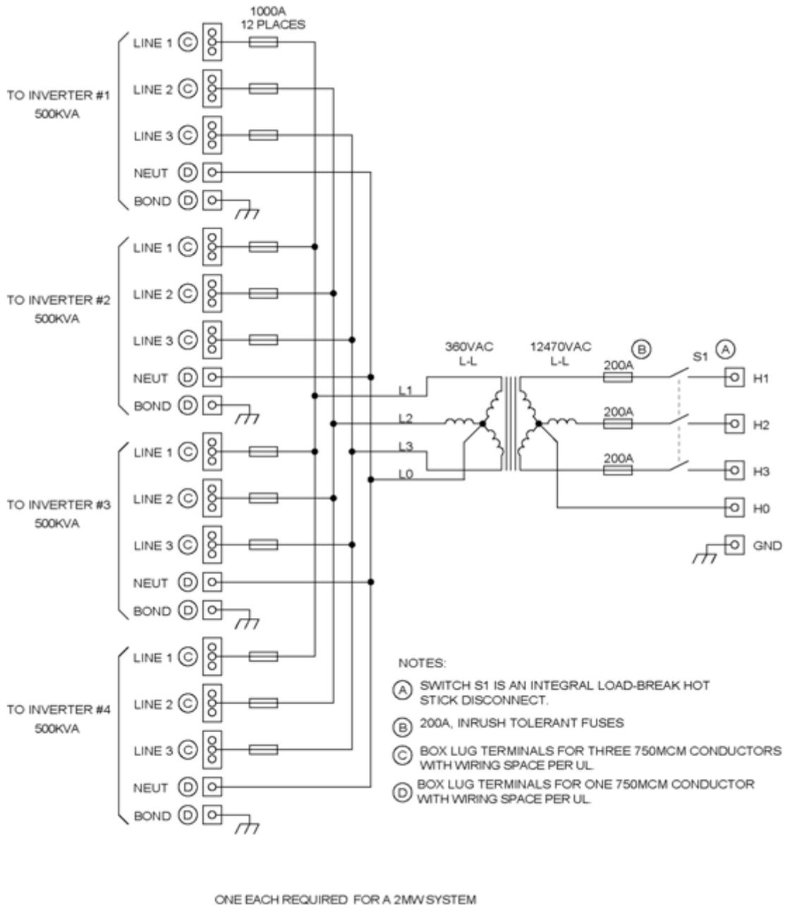
**Figure 9 - Solution #2, 2MVA Transformer Subassembly Schematic**
