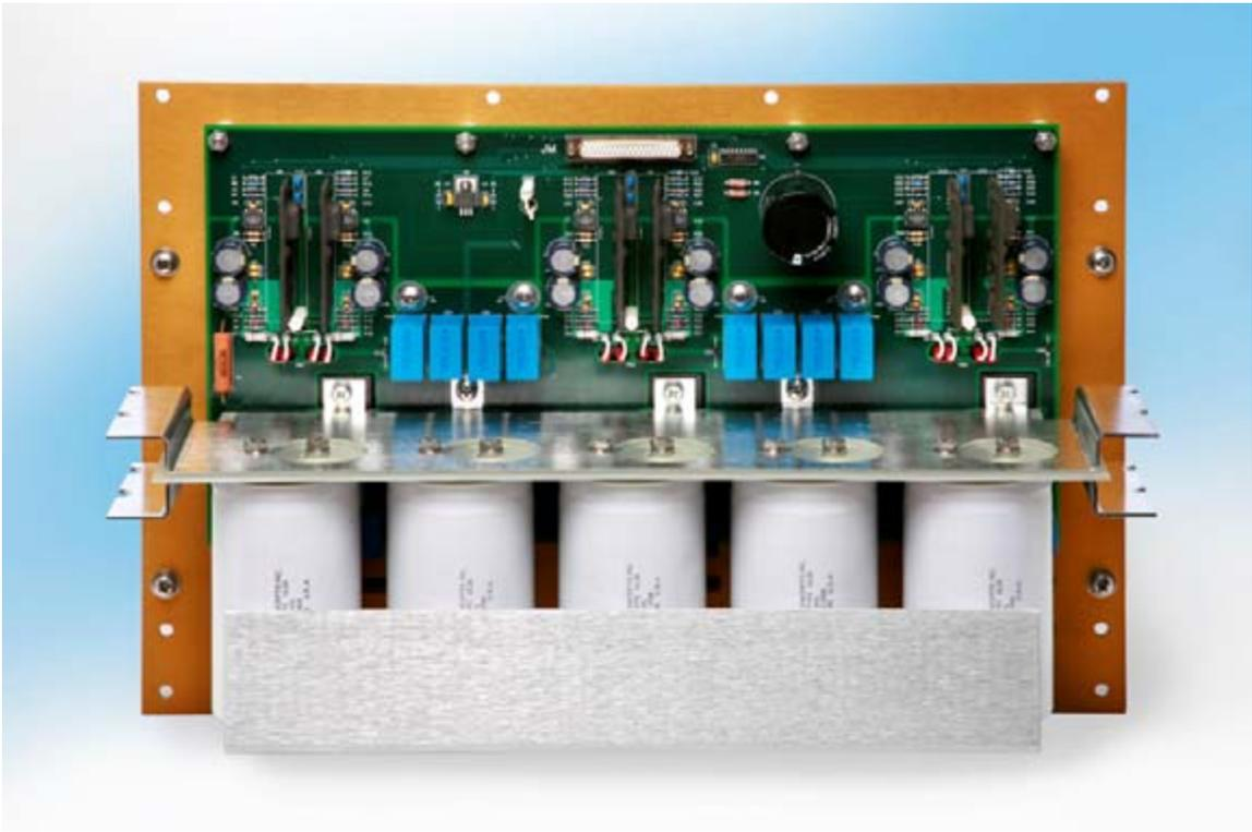
**Photograph 3 - Bridge Matrix Assembly, front**
