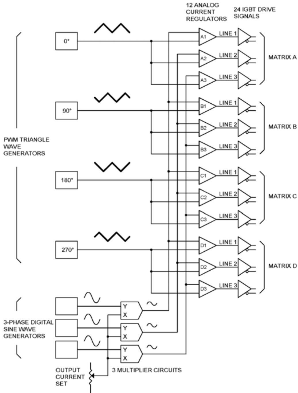
Figure 4 – Analog Control Board Regulation Circuits
