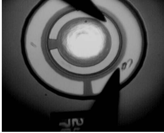
Figure 2.2. Top view microscope photograph of a partially fabricated photodiode being illuminated with an 850-nm laser spot inside the 70-um top metal aperture.
