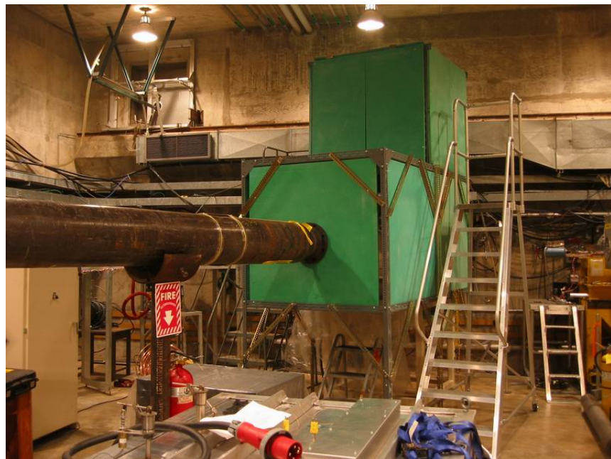
Fig. 42. The assembled experimental system showing the polyethylene shielding structure (green) surrounding the graphite heating system.
