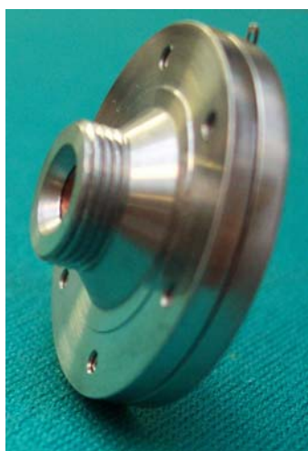
Fig. 2. Sample cell used to hold the Pu-Ga alloy samples in multiple containment.
