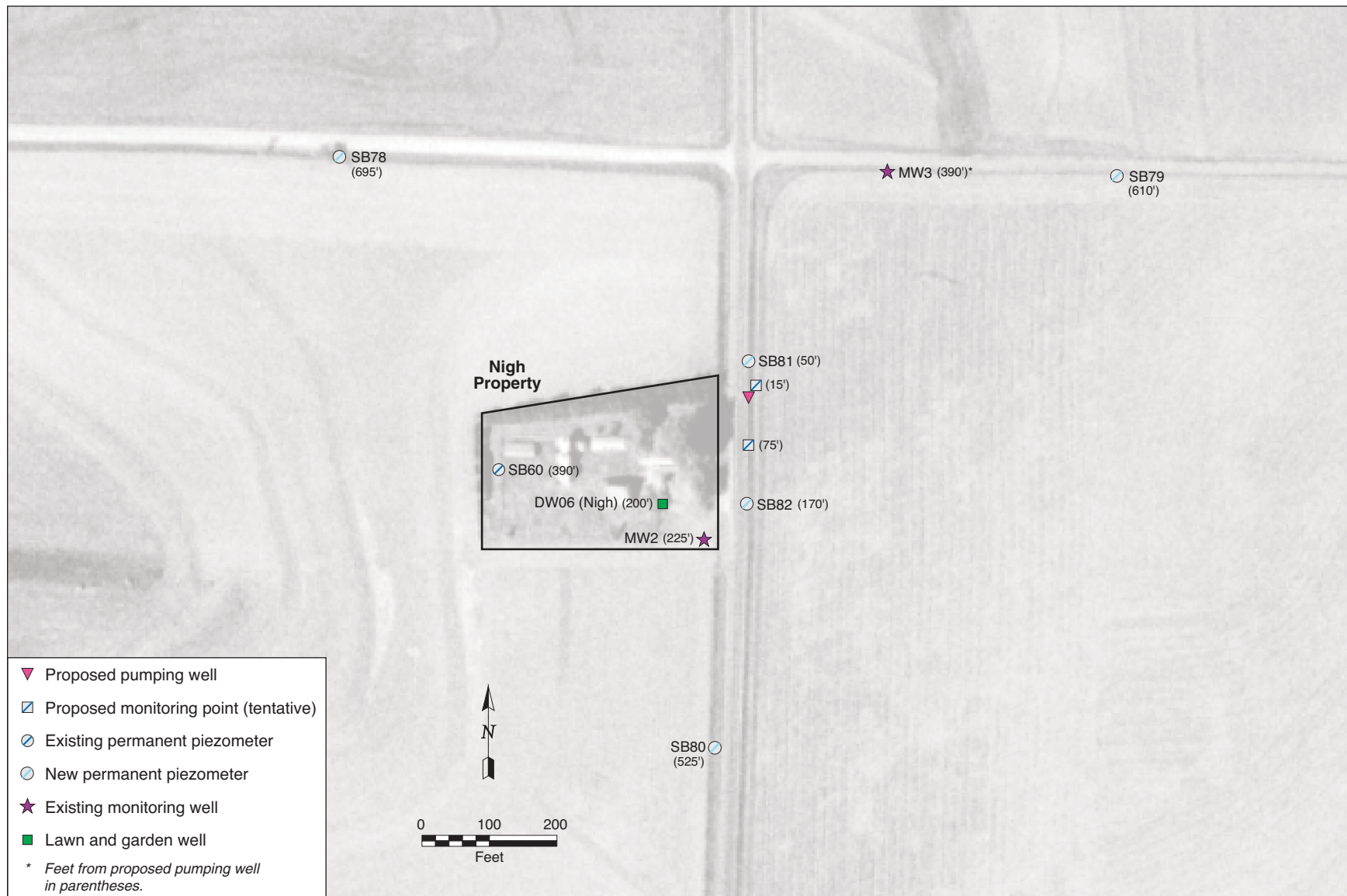
FIGURE 2.1 Proposed locations for a new pumping well and water level observation points (to be installed with the cone penetrometer) for proposed aquifer testing along the plume migration pathway northeast of the Nigh property at Everest.
