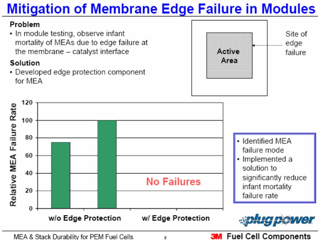
**Figure 15: Edge seal protection<sup>6</sup>**
