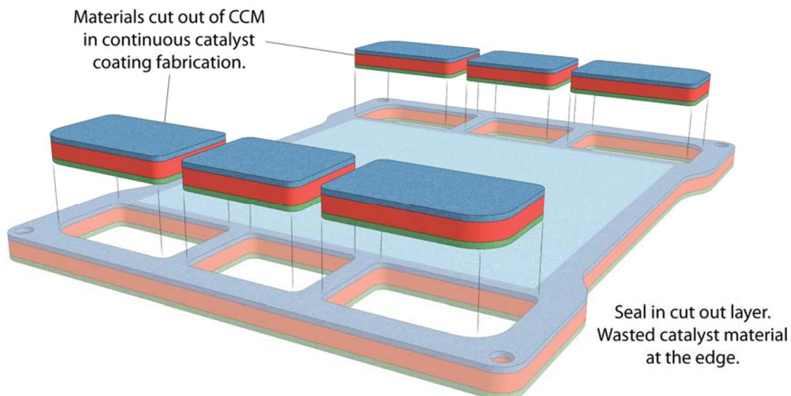
**Figure 7. Material loss in membrane manufacturing approach**
