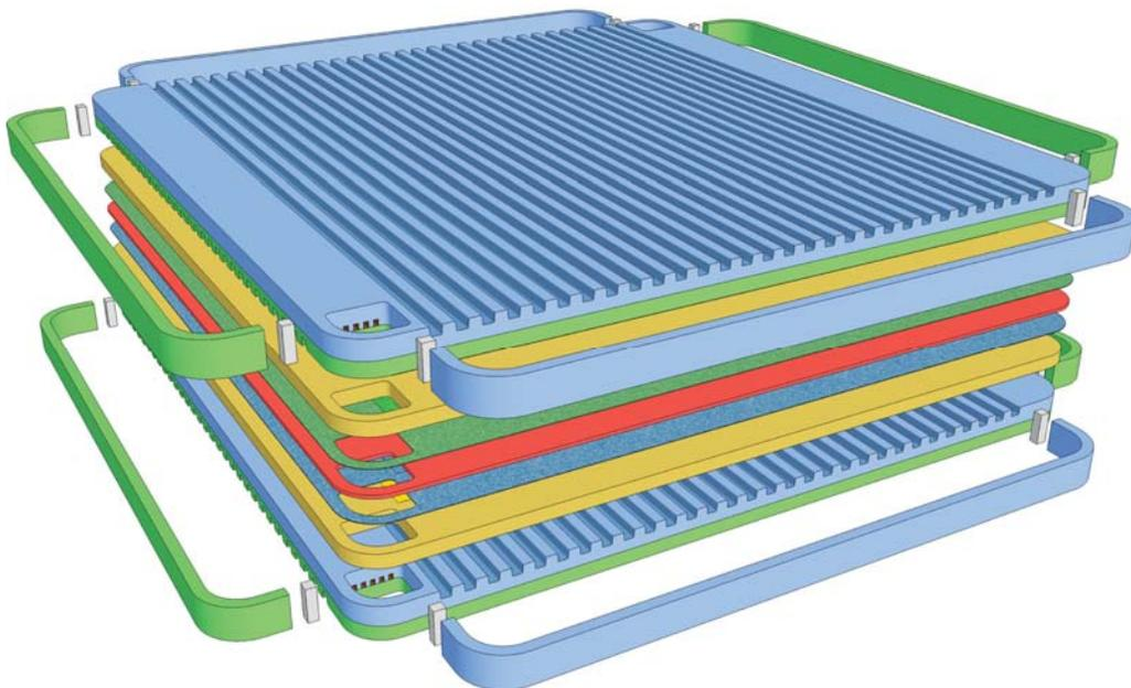
**Figure 6. Cell stack with a combination internal-external manifold**
