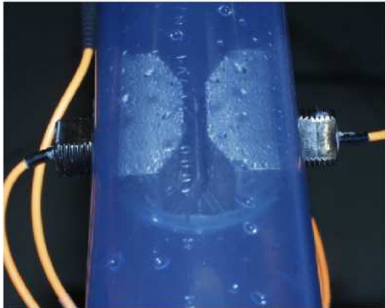
Figure 1.5: Near Infrared Sensor Mounted in Flow Loop
