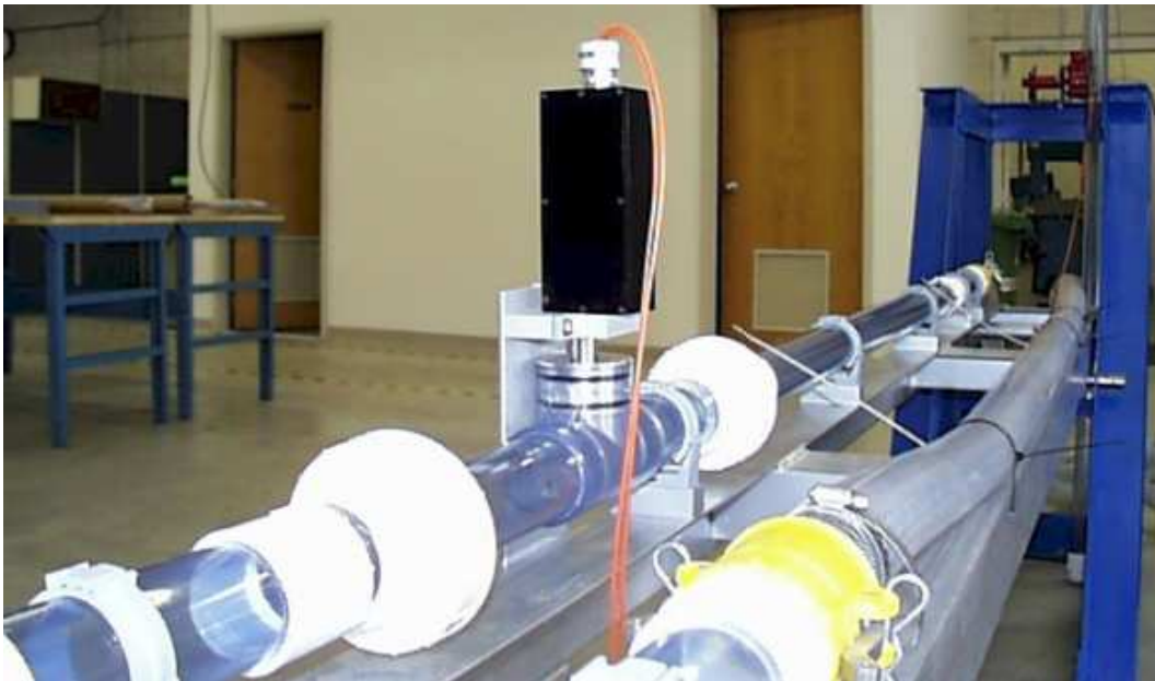
Figure 1.4: Fluorescence Probe Mounted on Adjustable Inclination Section
