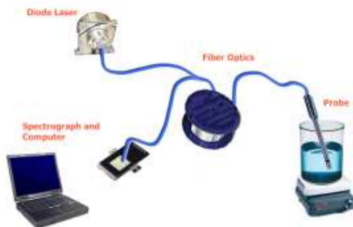
Figure 2.9: Instrumental arrangement for measuring fluorescence of crude oil and water mixtures
