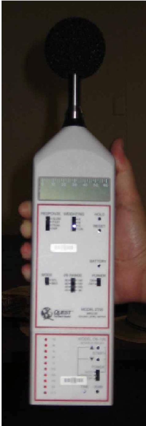
Figure 19: Sound intensity meter used for calibrating source level at receiver array.
