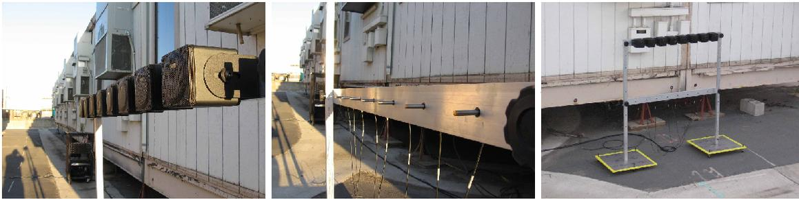
Figure 17: Time reversal array system of 8 speakers (left), 8 microphones (center), arranged in two horizontal arrays (right).
