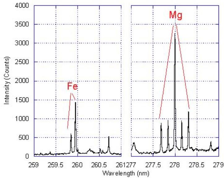
Figure 12 - LIBS Atomic Emission Lines from Fe and Mg from Molten Fiberglass
