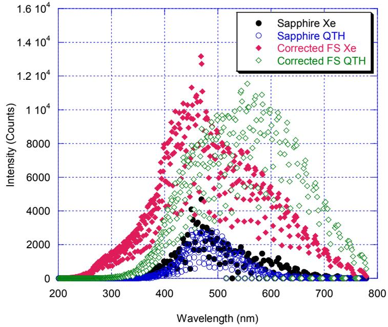
Figure 5 - Broadband Comparison of Sapphire and Fused Silica Fibers
