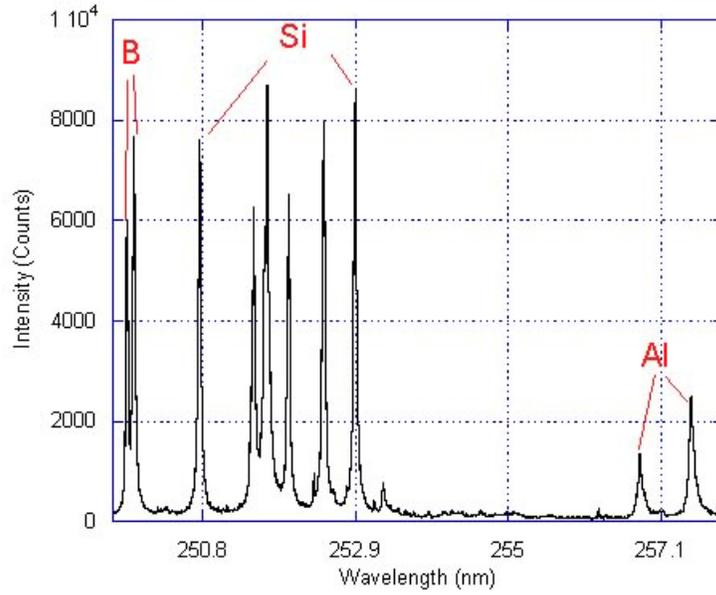
Figure 11 - LIBS Emission Lines from B, Si and Al in Molten Fiberglass
