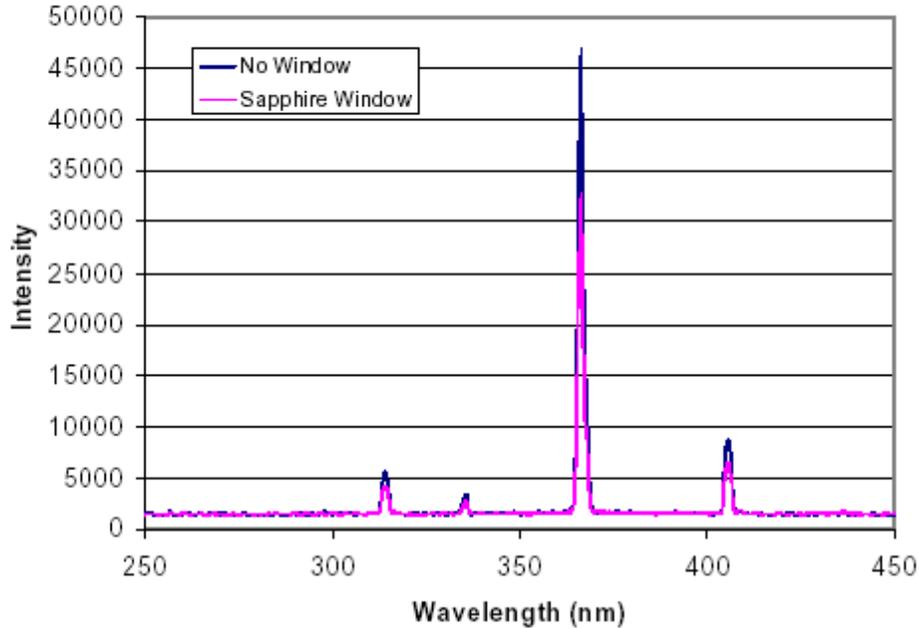
**Figure 4- Transmission of UV Source With and Without Sapphire Window**
