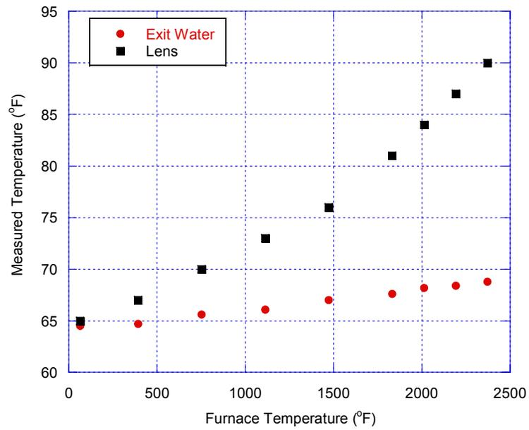
**Figure 9 - Results of LIBS Molten Glass Probe Cooling Test**
