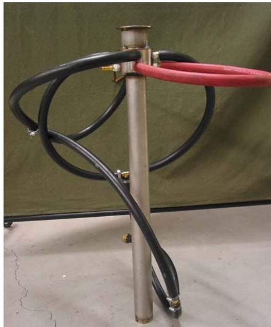
Figure 6 - LIBS Molten-Glass Sensor
