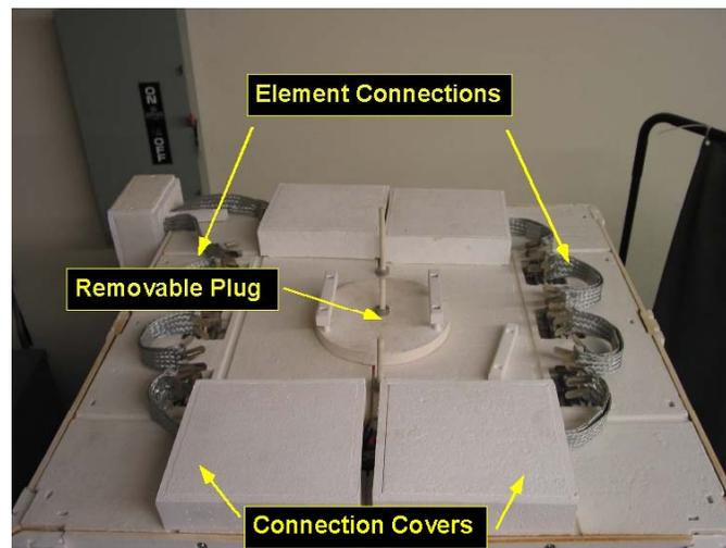
**Figure 16 - Top View of Connections and Hot Space**
