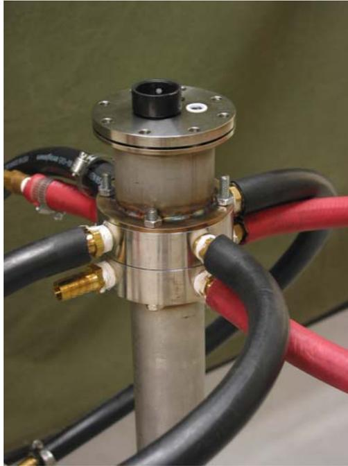
**Figure 7 - Closeup of LIBS Sensor**
