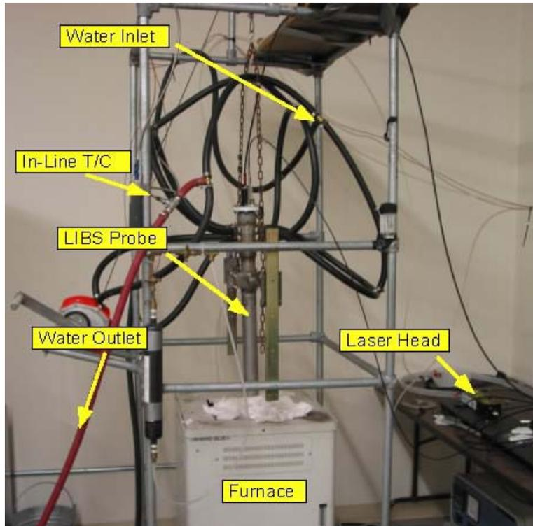
**Figure 8 - Laboratory Setup for LIBS Probe Cooling Test**
