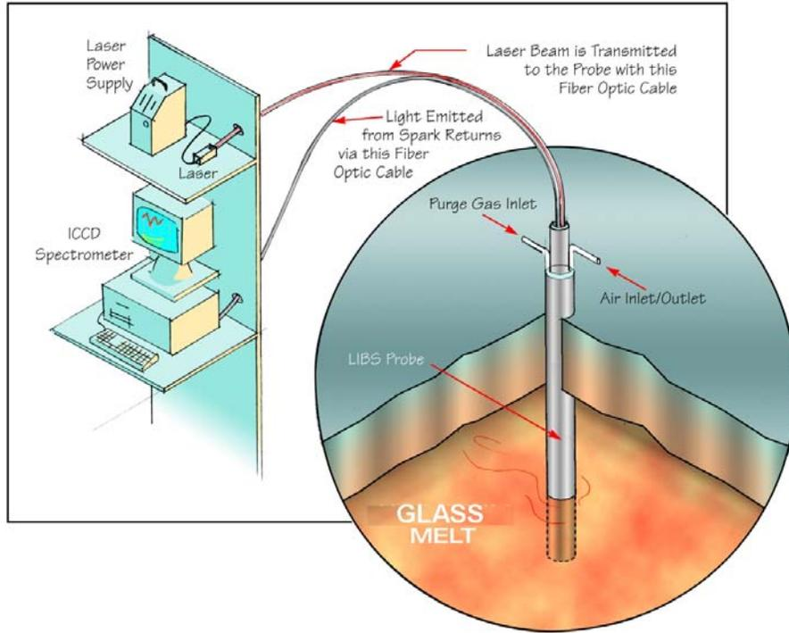
Figure 1 - Schematic of LIBS Probe for Molten Glass
