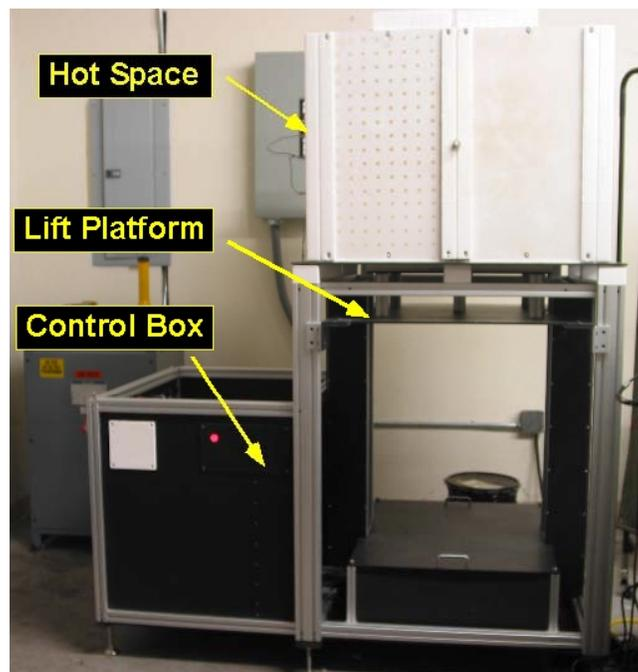
Figure 14 - Photograph of High Temperature Kiln
