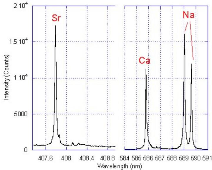
Figure 13 - LIBS Atomic Emission Lines from Sr, Ca and Na from Molten Fiberglass
