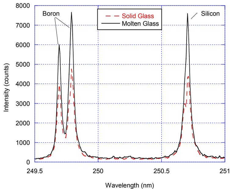
Figure 10 - Comparison of LIBS Spectra from Solid and Molten Glass
