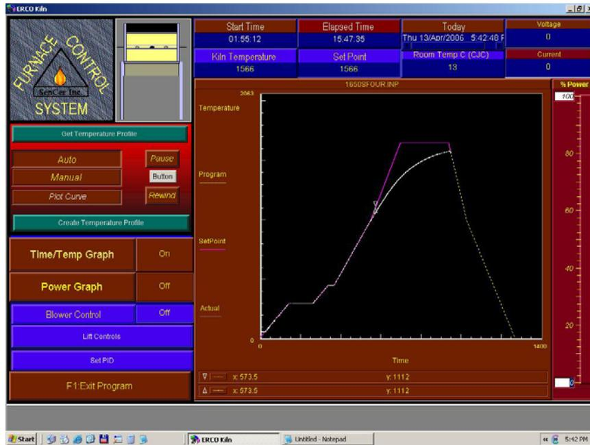
Figure 17 - Furnace Operator Control Screen
