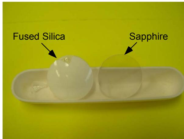
Figure 3 - Fused Silica and Sapphire Lenses after Exposure at 1500 C
