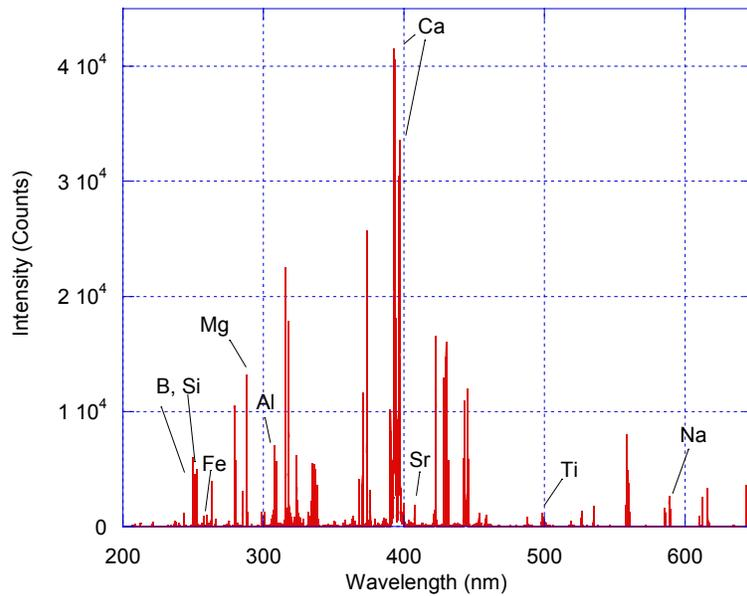
Figure 2 - Typical LIBS Spectrum from Solid Fiberglass
