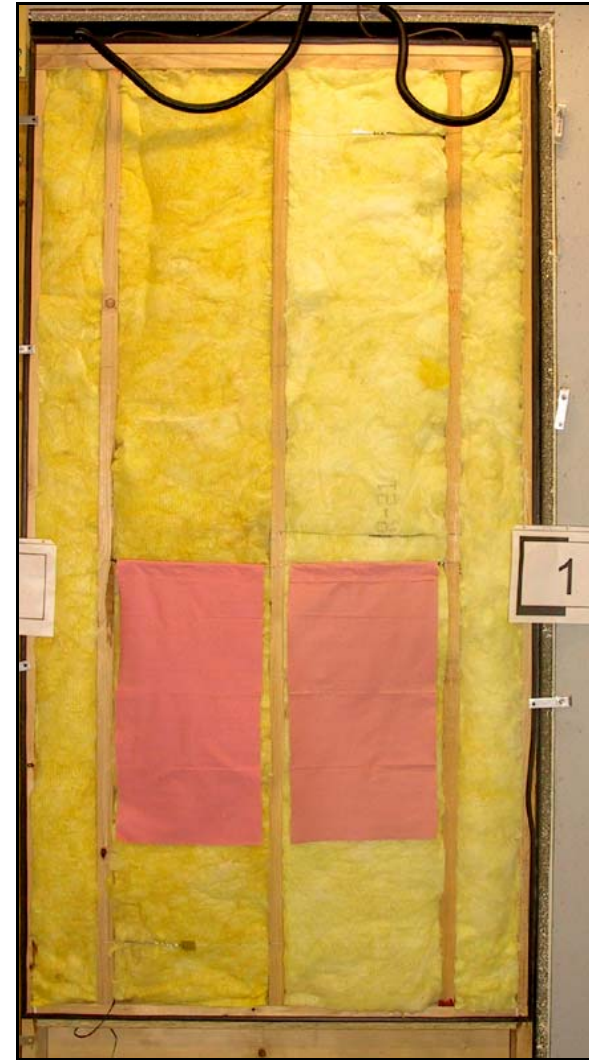
5 Test Wall Cavity with insulation and absorbent material
