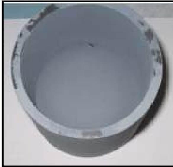
Figure 7. Coated graphite crucible. Used in MG3-107. It was found that the adherence of the coatings could be affected by rate of temperature ramping during the firing, as well as the atmosphere, and the previous processing of the crucible. A standard approach was developed that allowed reproducible coatings to be applied that allowed the crucible to be reused. If the process was not followed, the coating was uneven and not always suitable.
