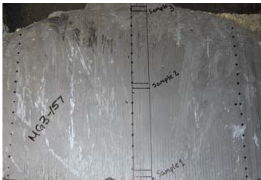
Figure 10. Results from slagging run MG3-157. This run contained 20 kg of upgraded metallurgical silicon. The locations for sample 1 and sample 3 are shown. These analyses are shown in Table 6.
