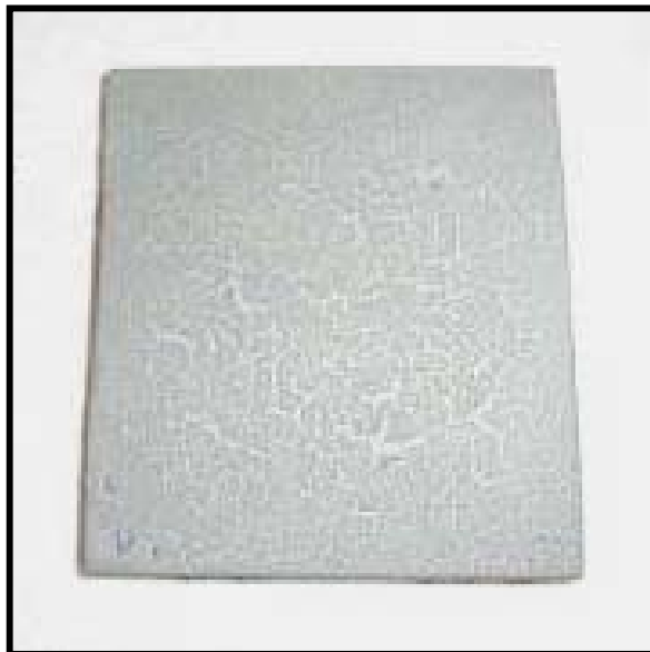
Figure 8. 4"x4" coupon coated and processed in a normal experimental run. Coating was cracked but adhered. It was discovered that the rates at which the various coatings were heated and baked impacted their ability to adhere and form continuous sheets.
