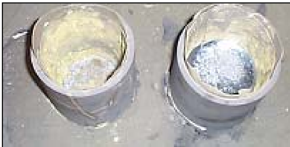
Figure 9. Liners in two crucibles. The crucible on the left has lost all of its silicon due to wicking. The crucible on the right contained its silicon under the exact same conditions.
