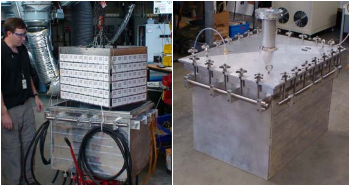
Figure 5. Internal enclosure of test chamber with heat flux measuring sensors being placed in the external enclosure of test chamber (left). Completed test chamber for the large calorimeter (right).
