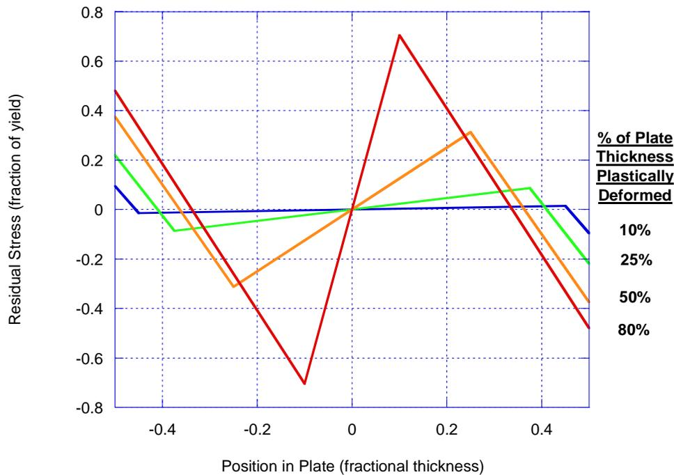
**Figure 24. Comparative Residual Stress Profiles.**
