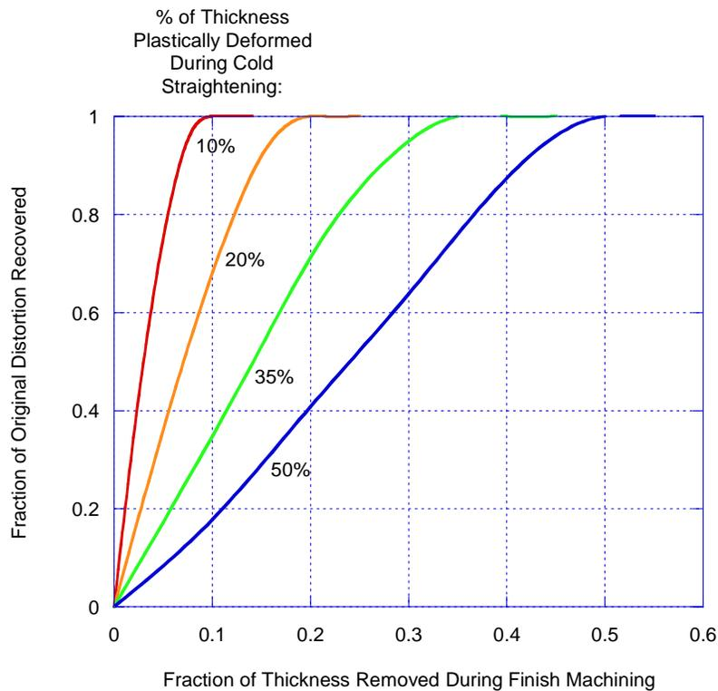
**Figure 27. Returning Distortion When Previously Cold Straightened Plates Are Finish Machined.**
