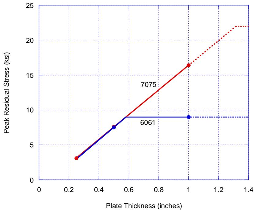
**Figure 5. Residual Stress Increases with Increasing Thickness Up to As-Quenched Yield Strength.**
