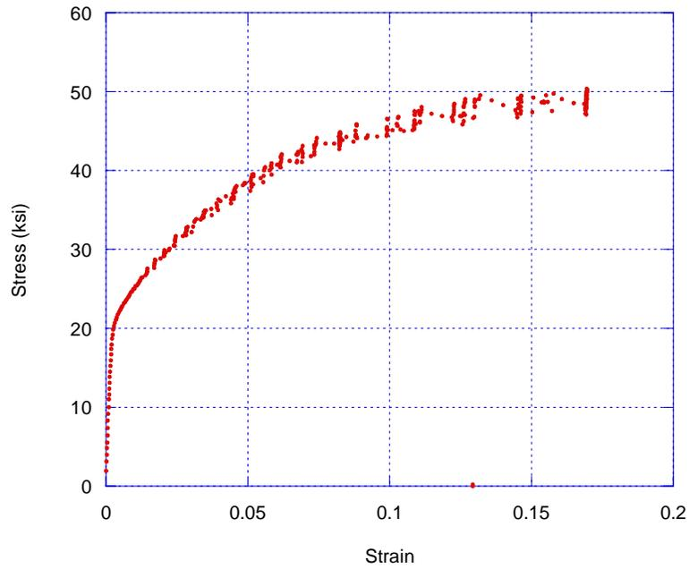
**Figure 3. Tensile Stress-Strain Curve of As-Quenched 7075.**
