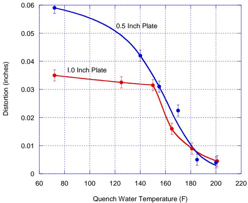
**Figure 17. Effect of Quench Water Temperature and Thickness on Distortion (6061-T6).**
