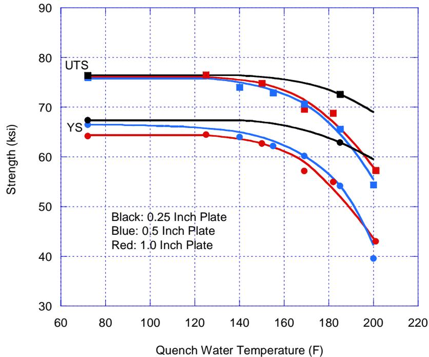
**Figure 21. Effect of Quench Water Temperature and Thickness on Yield and Ultimate Tensile Strength (7075-T73).**
