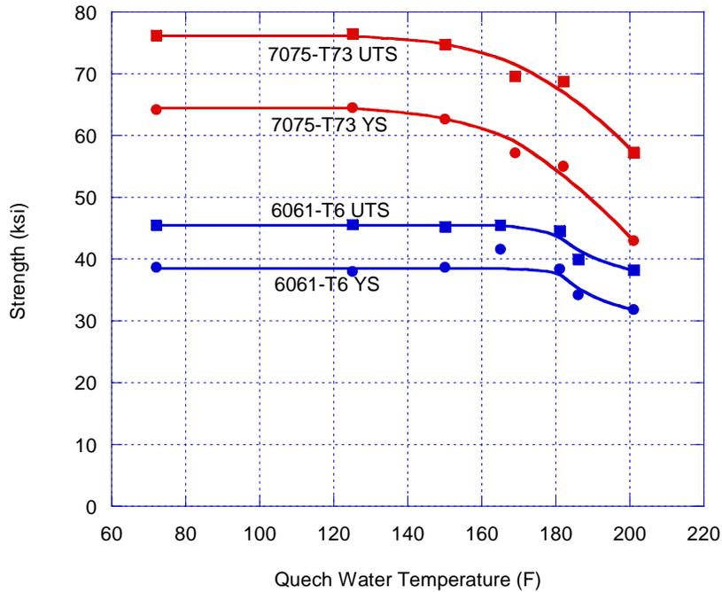
**Figure 15. Effect of Quench Water Temperature on Yield and Ultimate Tensile Strength (7075-T73 and 6061-T6, 1 Inch Thick).**
