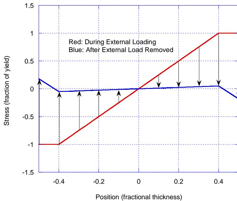
**Figure 23. Residual Stress Development During Cold Straightening.**
