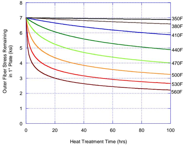
**Figure 8. Calculated Effects of Overaging Temperature and Time on Peak Residual Stresses (6061).**
