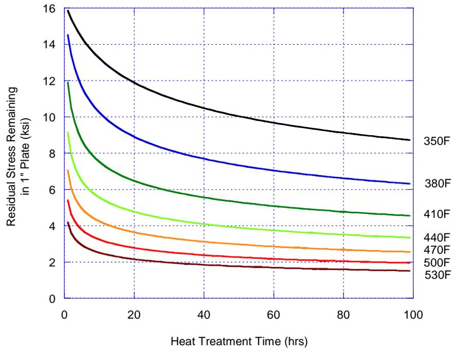
**Figure 9. Calculated Effects of Overaging Temperature and Time on Peak Residual Stresses (7075).**
