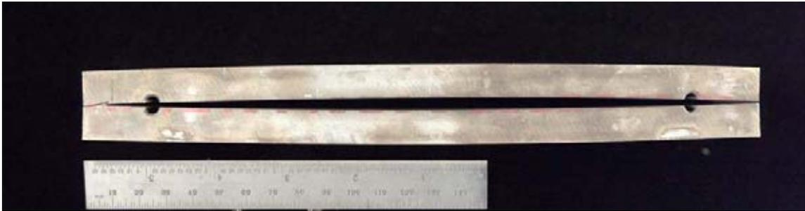
**Figure 1. Distortion in 7075-T6 Plate Electro-Discharge Machined Along Its Centerplane.**
