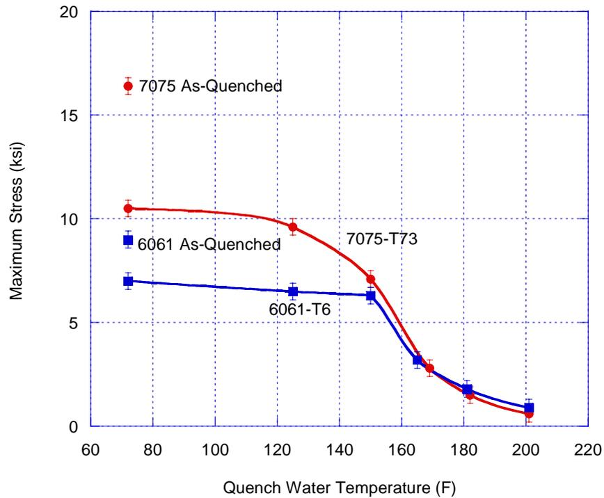
**Figure 14. Effect of Quench Water Temperature on Peak Residual Stress (7075-T73 and 6061-T6, 1 Inch Thick).**
