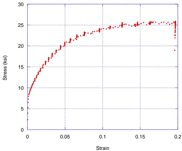
**Figure 4. Tensile Stress-Strain Curve of As-Quenched 6061.**
