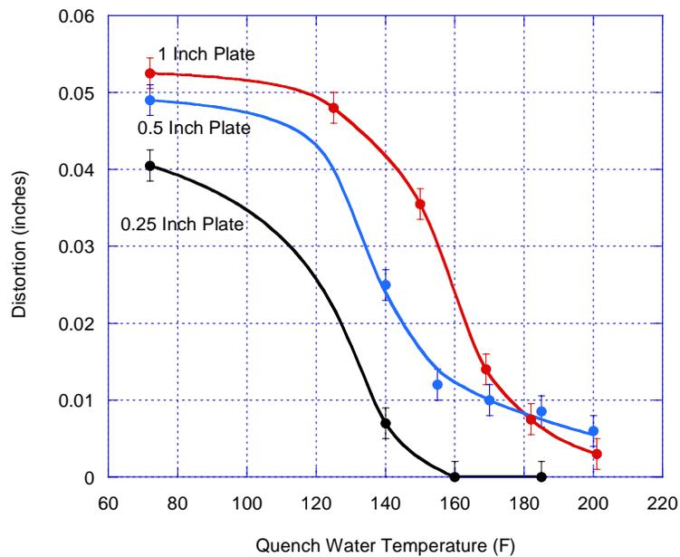
**Figure 20. Effect of Quench Water Temperature and Thickness on Distortion (7075-T73).**
