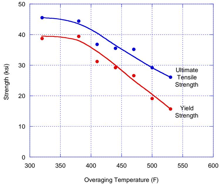
**Figure 10. Effect of Overaging for 18 Hours on Yield Strength and Ultimate Tensile Strength (6061).**
