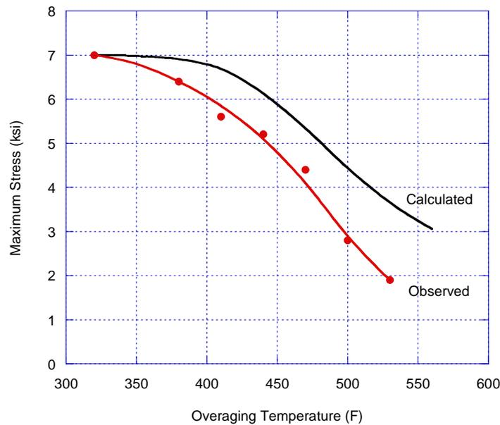
Figure 6. Peak Residual Stresses After Overaging 18 Hours (6061).
