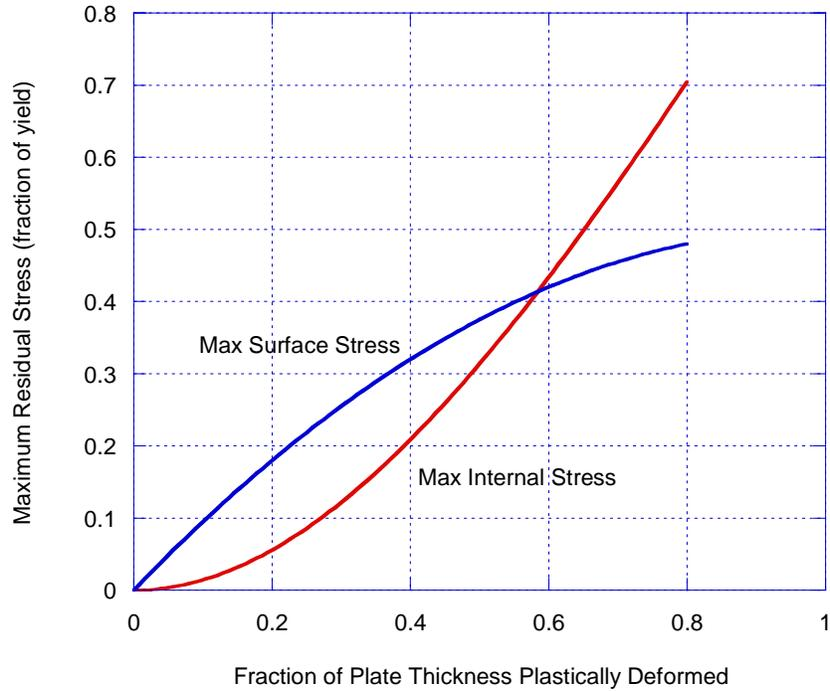
**Figure 25. Maximum Surface and Internal Residual Stresses.**
