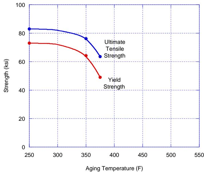
**Figure 11. Effect of Overaging for 18 Hours on Yield Strength and Ultimate Tensile Strength (7075).**
