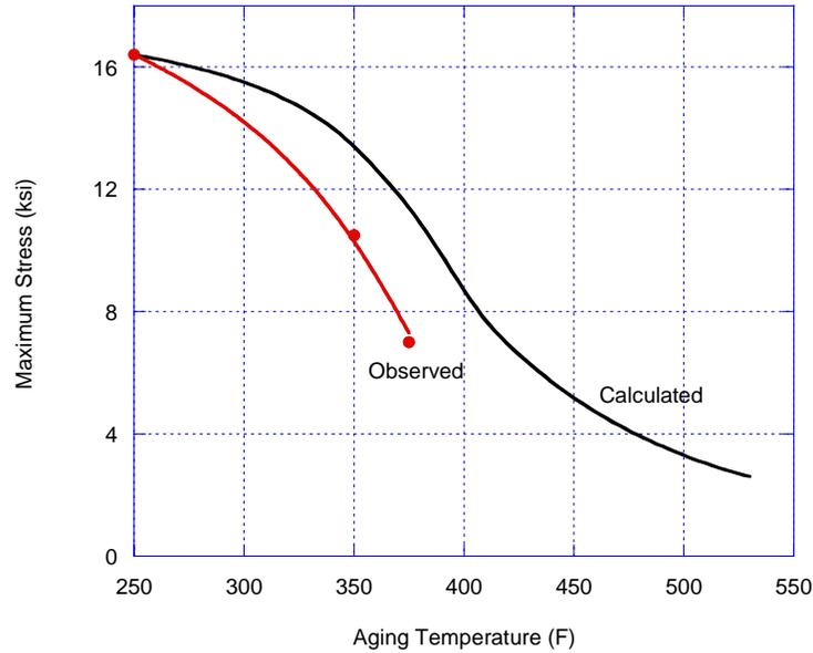
**Figure 7. Peak Residual Stresses After Overaging 8 Hours (7075).**
