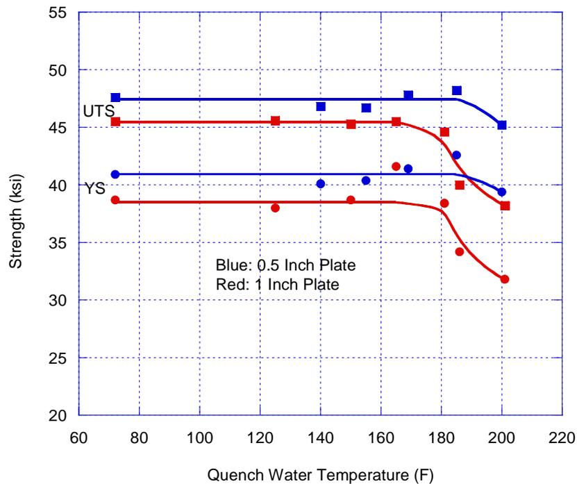
**Figure 18. Effect of Quench Water Temperature and Thickness on Yield and Ultimate Tensile Strength (6061-T6).**
