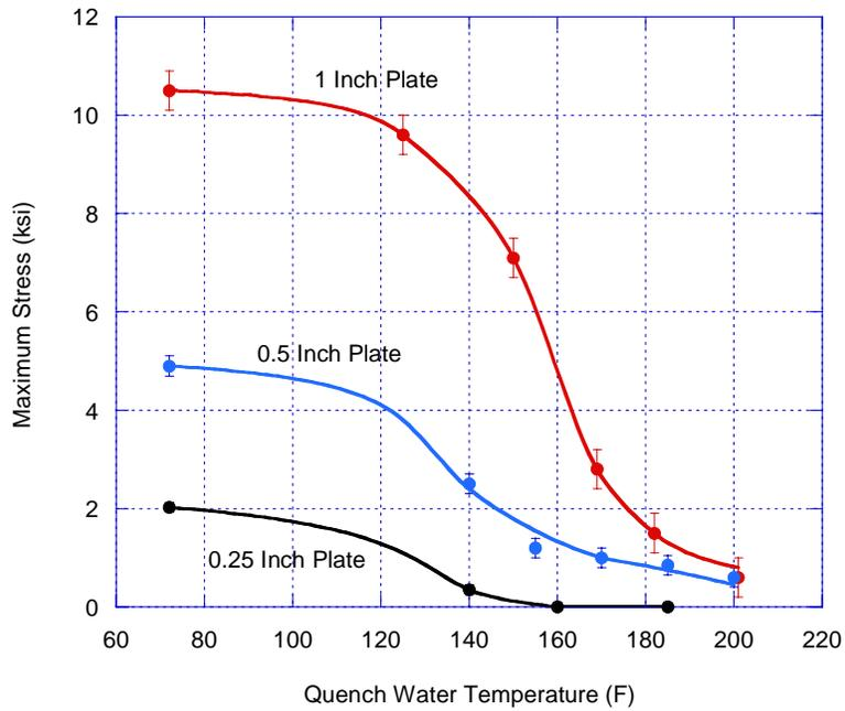
**Figure 19. Effect of Quench Water Temperature and Thickness on Peak Residual Stress (7075-T73).**
