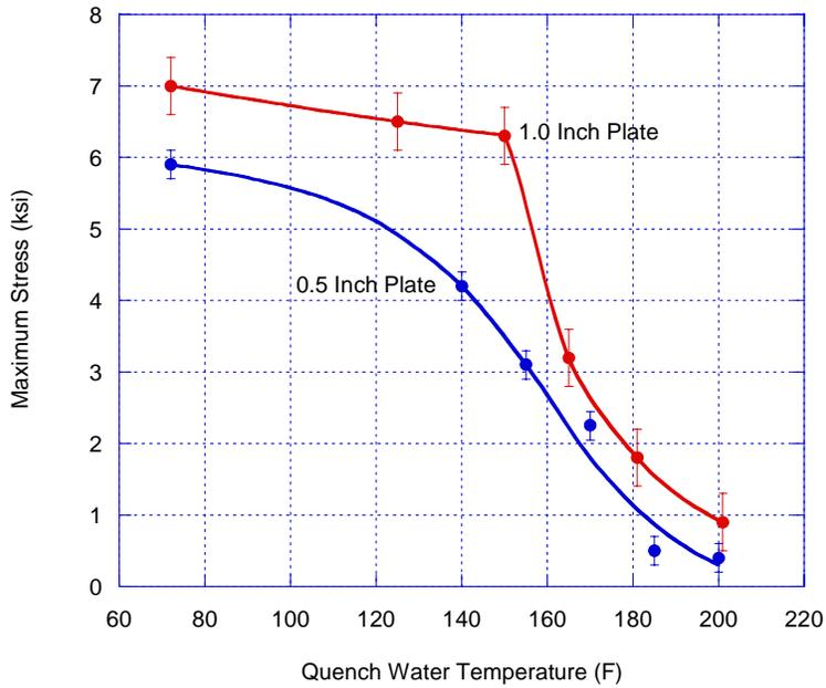
**Figure 16. Effect of Quench Water Temperature and Thickness on Peak Residual Stress (6061-T6).**
