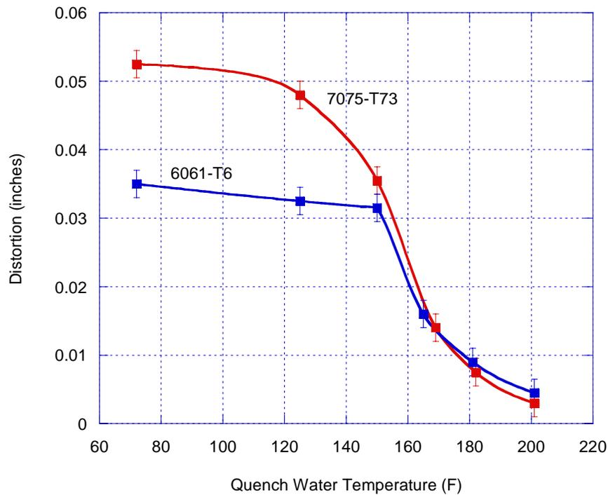
**Figure 13. Effect of Quench Water Temperature on Machining Distortion (7075-T73 and 6061-T6, 1 Inch Thick).**
