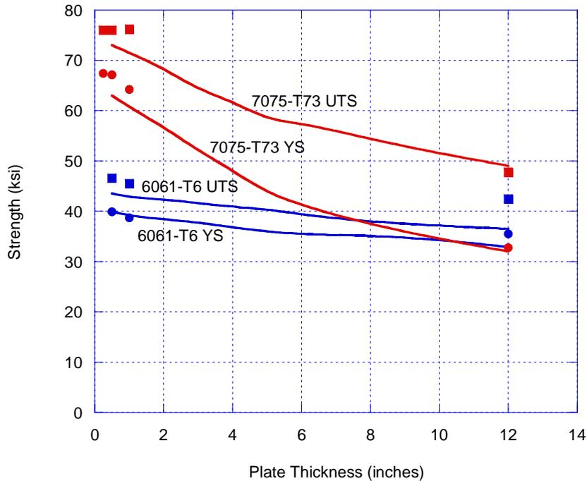
**Figure 12. Effect of Plate Thickness on Yield Strength and Ultimate Tensile Strength (7075-T73 and 6061-T6).**
