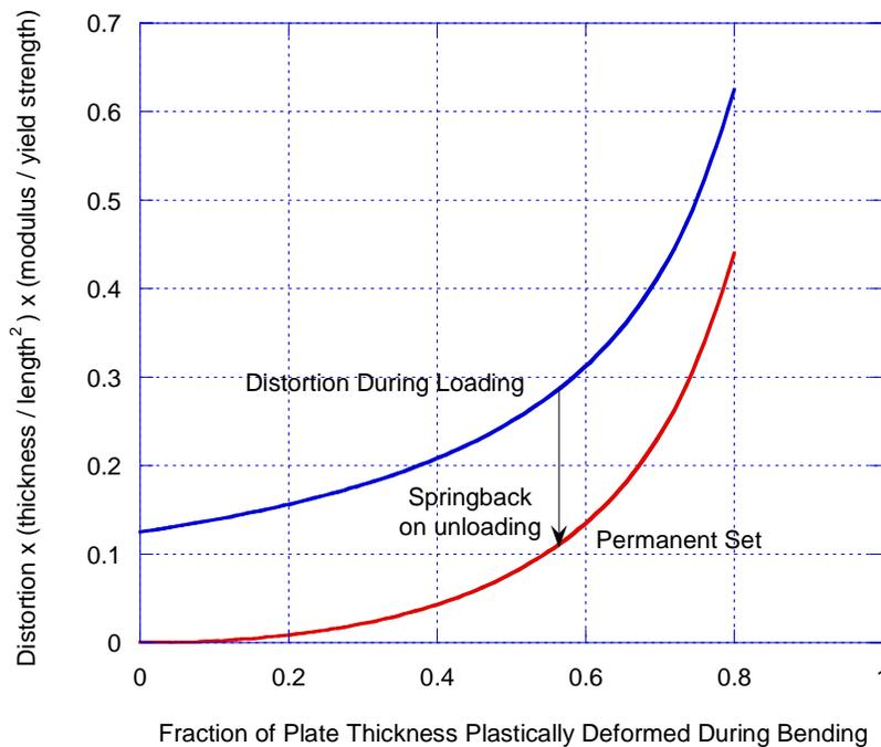
**Figure 26. Deflections During and After External Loading.**
