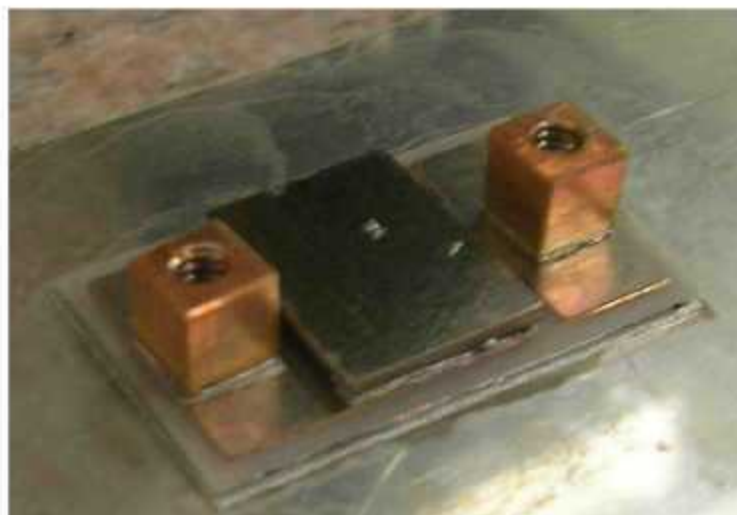
Fig. 9. A prototype flip-chip package.
