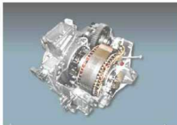
Figure 2-5. Camry HEV Transaxle Schematic and Cutaway View.
