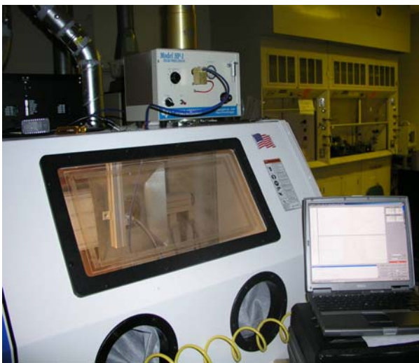
Automated micro blasting system, left and 500u micro-blasted via through pyrex
