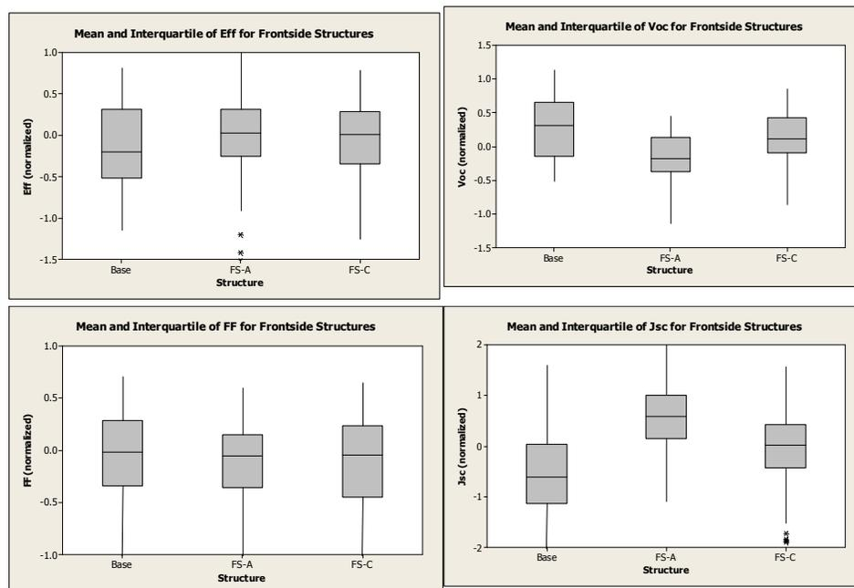
**Figure 3: Distribution of post-stress Efficiency, Voc, FF and Jsc for two front side structures plus Base.**
