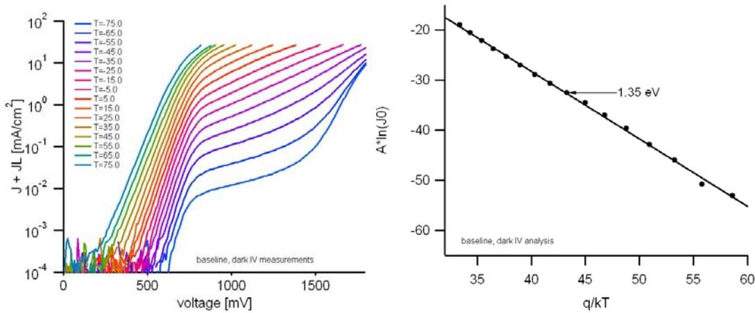
**Figure 11: (left) dark IV measurements at various temperatures and (right) extraction of the recombination energy.**
