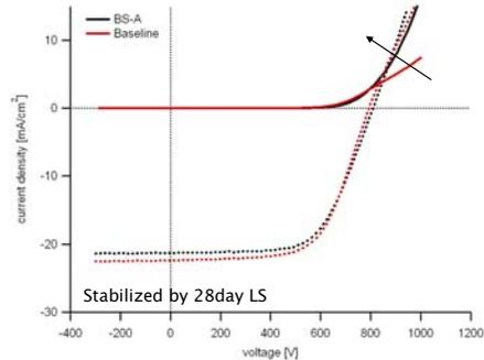
**Figure 7: Comparison of the light-dark crossover points from the Base and BS-A structures indicates that the BS-A back contact has qualitatively lower resistance than that of the Base structure.**
