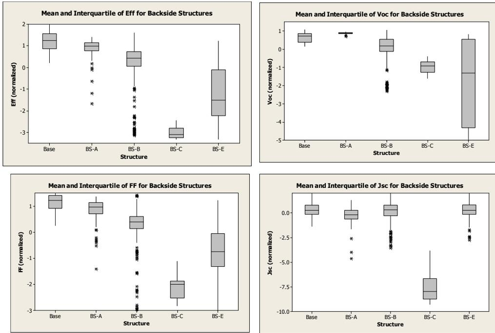
**Figure 4: Distribution of initial Efficiency, Voc, FF and Jsc for four backside structures plus Base.**
