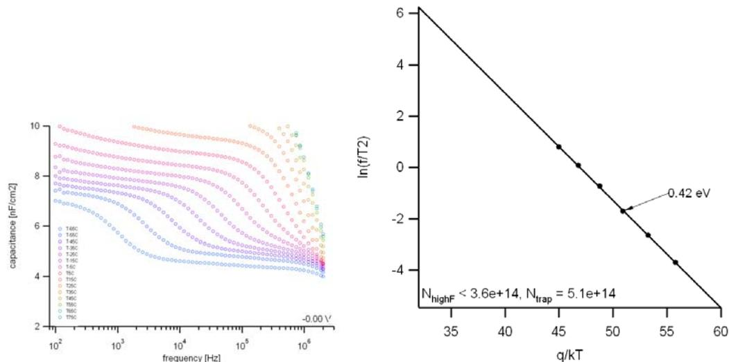
**Figure 13: C-f measurements on baseline sample at zero bias and data plotted for determination of the trap level energy.**
