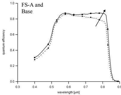
**Figure 6: Comparison of quantum efficiency of the FS-A and Base structures indicates qualitative differences responsible for the improved Jsc of FS-A.**
