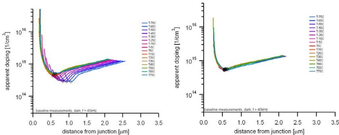
Figure 12: (left) dark and (right) illuminated C-V measurements.
