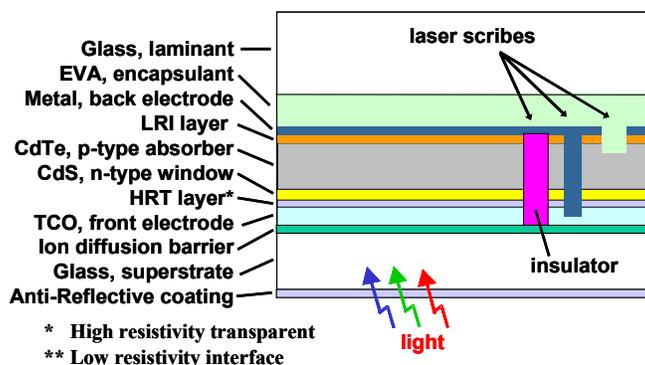
**Figure 1: Schematic of CdTe/CdS PV module showing monolithic interconnect.**
