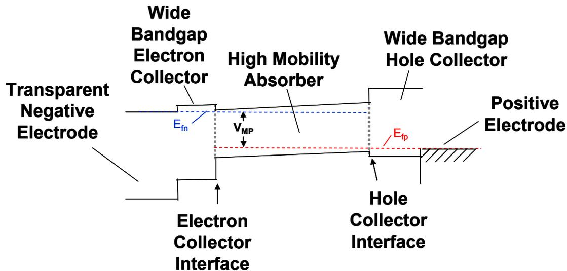
Figure 14: Idealized p-i-n structure conceptual band diagram – a) in the dark with zero bias and b) under illumination at maximum power point.
