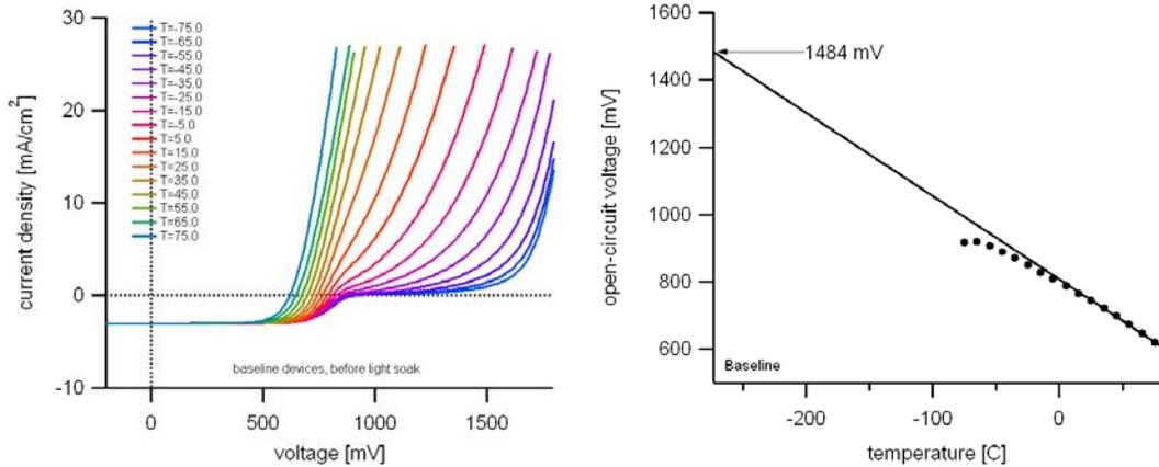
**Figure 10: (left) baseline IV measurements (not 1 sun), and (right) extrapolation of Voc vs temperature to zero Kelvin.**
