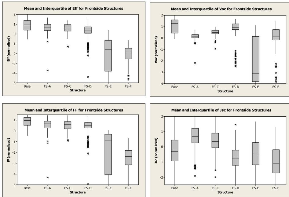
**Figure 2: Initial performance of five alternative front side structures plus the Base structure. Data are expressed in normalized units (subtract mean and divide by standard deviation).**
