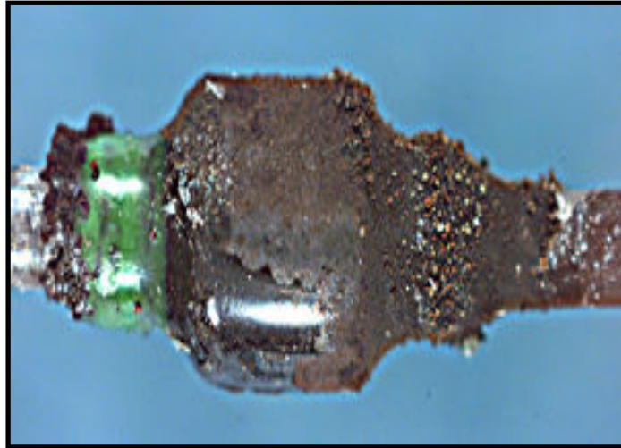
Figure 12. Sulfidation of a copper-containing braze in a zener diode (Braithwaite et al. 2003)
