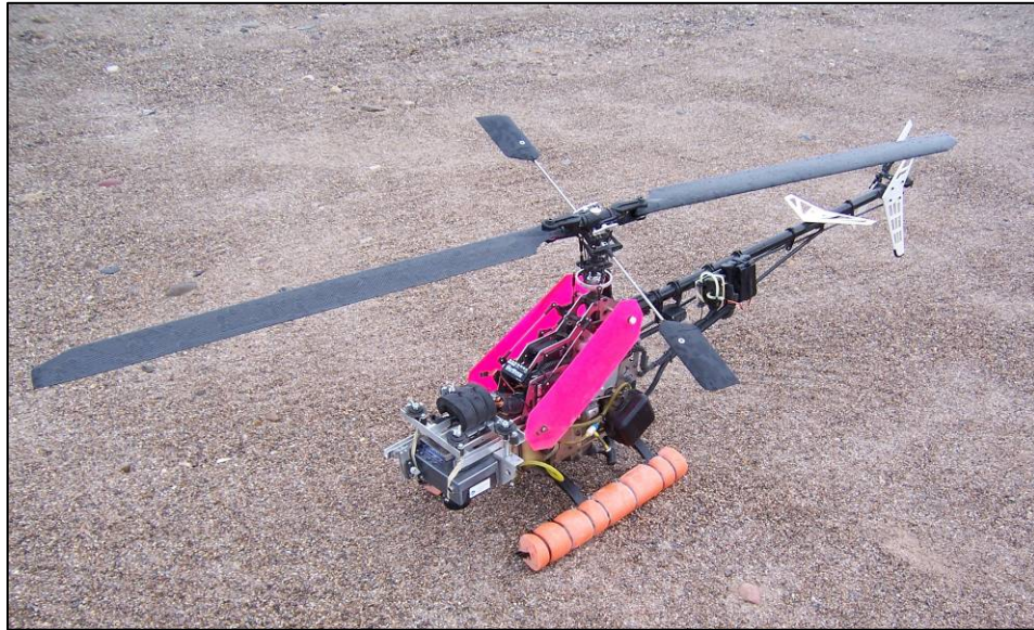
Fig. 16 The Predator Gasser radio control helicopter with the ADC2 camera mounted on the front of the RCH. The bright pink panels make it easier to see the RCH orientation in flight and the spongy orange skids also aid in visual orientation as well as softer landings. The altimeter is mounted mid-way between the engine and tail on the fuselage.
